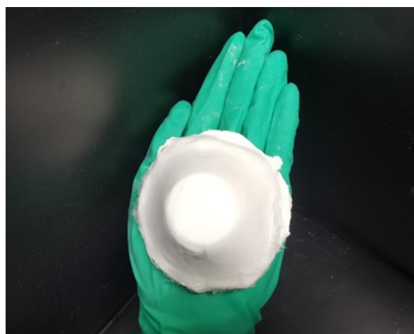
Figure S6. The precursor of N-TiO 2 CNSs with a diameter of 7.5 cm and a thickness of 3.5 cm.
