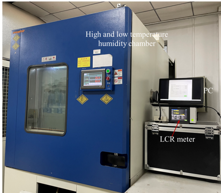
Fig.S14. The temperature and humidity resistance test platform.
