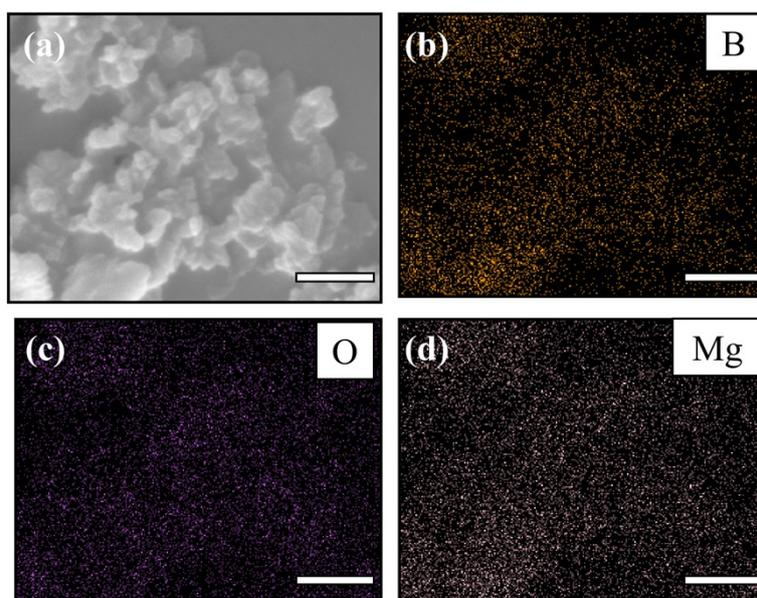
**Figure S1.** (a) SEM image of Mg-BNSs. (b-d) EDX mapping of Mg-BNSs.
