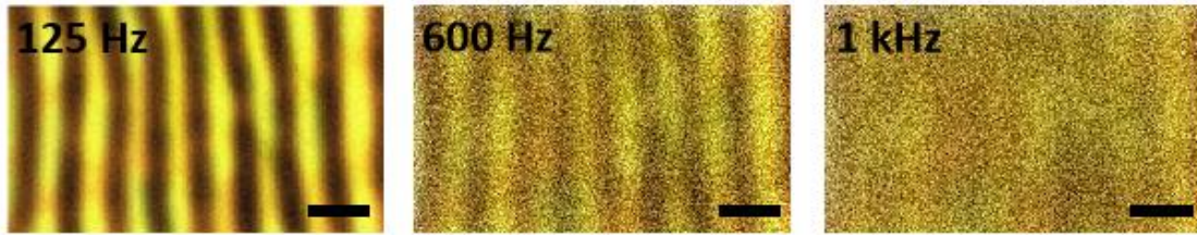
Figure S2. The Fe 3 O 4 -nanoparticle based MFM image of FePt perpendicular magnetic recording medium. The black bars represent 100 nm.
