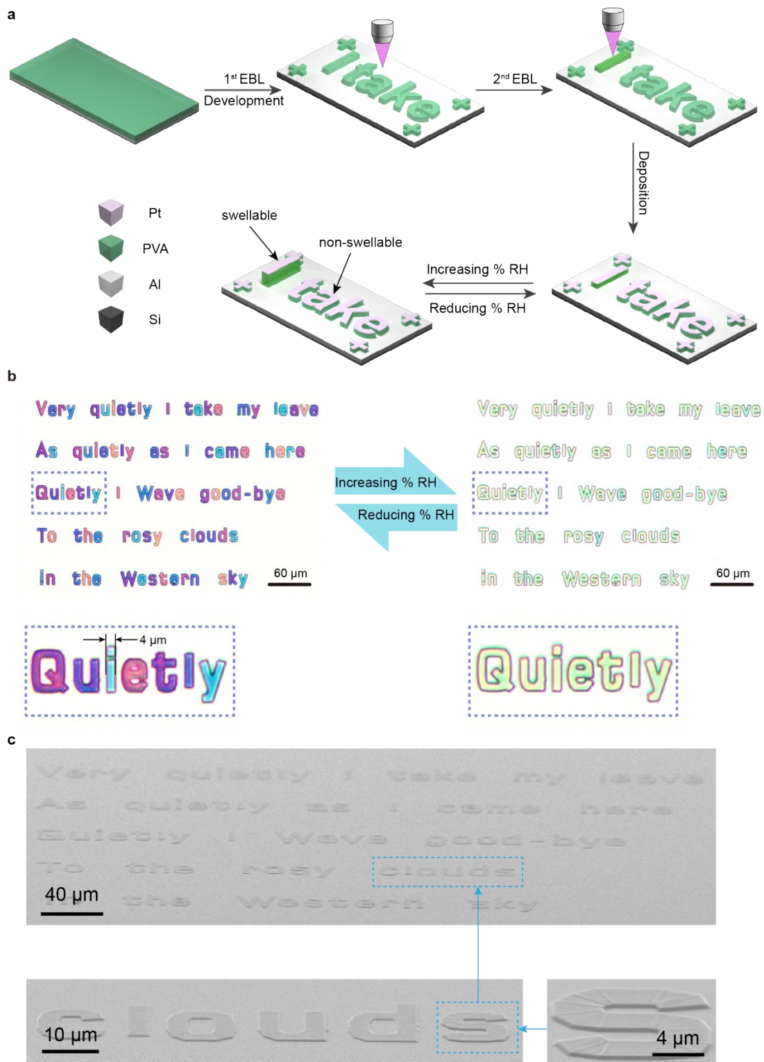
Figure S9. (a) Fabrication process flow of the double exposure structure. (b) Optical images of the excerpt of the poem Saying Good-bye to Cambridge Again without the second exposure, which is tunable by switching humidity between 40 and 100% RH. (c) SEM images of the corresponding structures.
