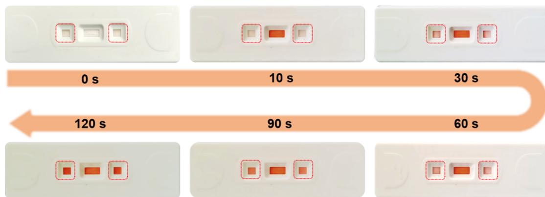
**Fig. S14** The solution flow on the LFTS sensing platform.
