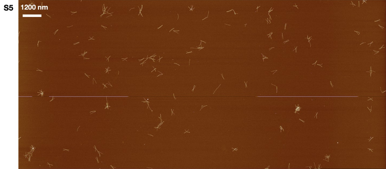
Figure S5. AFM images of two-folding geometry. Excluding non-desired monomer, dimer, and non-specific aggregations, the percentage of trimer with two-folding geometry is at least 70% (Statistics was obtained from over 500 DNA origami, the AFM image in the figure is only a representative one). It is safe to set the threshold to be 50% to read the output to be “1”.
