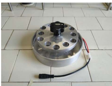
MultiVial Photoreactor: home-made, custom-designed; internal diameter 14.4 cm with 12 vial holes. Blue LED stripe 465 nm, 24 \text{ W/m} , ORBLUF52120812, 44 cm.
