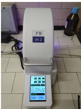
PennPhD Photoreactor m2 with 455 nm LED ( 3.4 \text{ W/cm}^2 ). K-type temperature probe.
