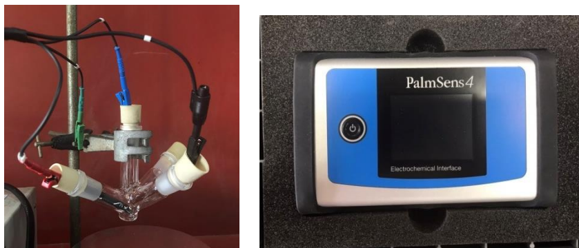
Fig. S1 Cyclic voltammetry experiment set up.
