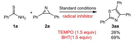
To a 15 mL sealed tube containing a magnetic stir bar were added benzothioamide (1a, 0.3 mmol, 1.5 equiv.), 2,3-diphenyl-2*H*-azirine (2a, 0.2 mmol, 1.0 equiv.), radical inhibitor (1.5 equiv.). HClO<sub>4</sub> (2.3  $\mu$ L, 0.04 mmol, 0.2 equiv.) was washed down by 1,2-dichloroethane (DCE, 2.0 mL) and the substrates were dissolved. After stirred for 16 h
