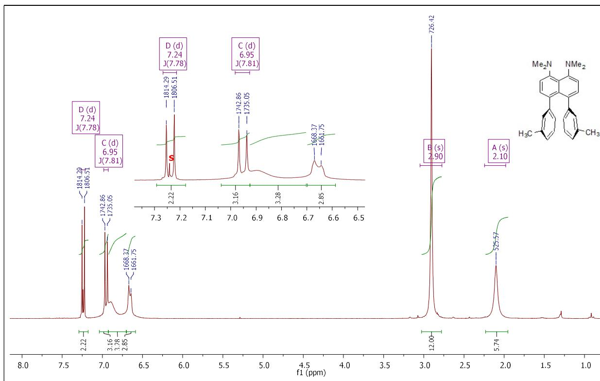
**Fig. S27.**  $^1\text{H}$  NMR spectrum of compound **3b** (250 MHz,  $\text{CDCl}_3$ ).
