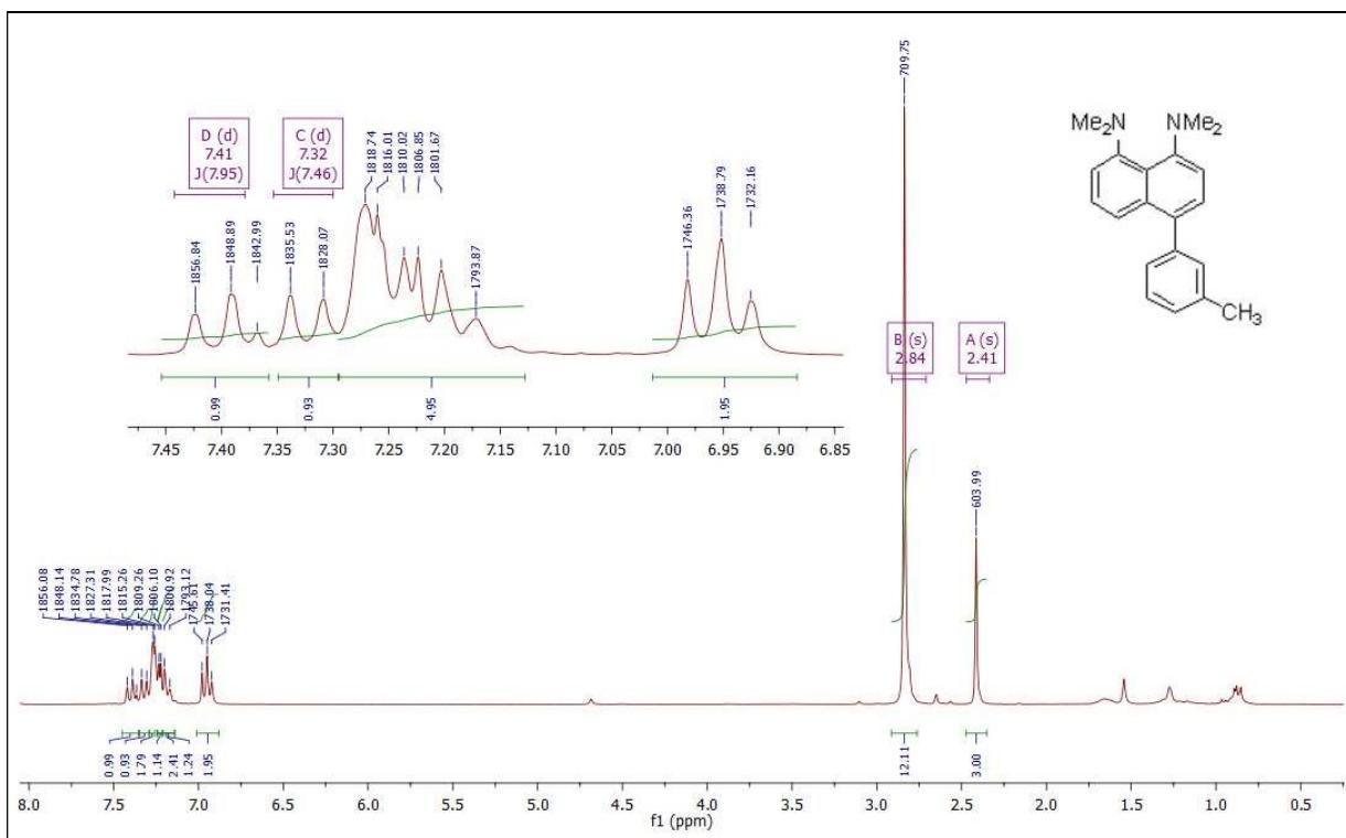
**Fig. S5.**  $^1\text{H}$  NMR spectrum of compound **5c** (250 MHz,  $\text{CDCl}_3$ ).
