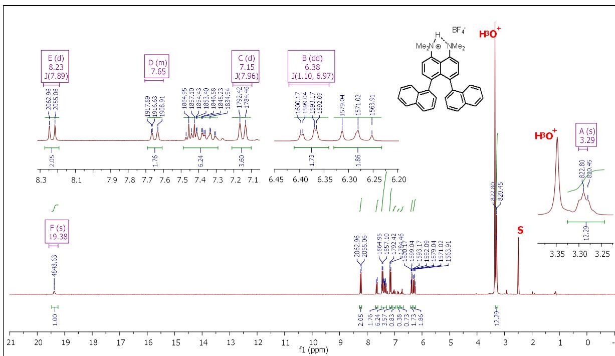
Fig. S45.  $^1\text{H}$  NMR spectrum of compound  $3\text{c}\cdot\text{HBF}_4$  (250 MHz,  $\text{DMSO-d}_6$ ).
