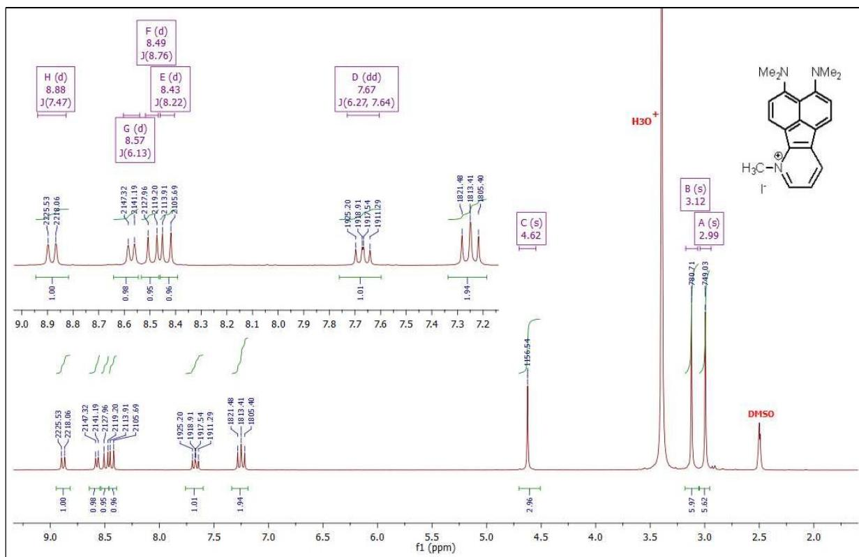
**Fig. S39.**  $^1\text{H}$  NMR spectrum of compound **12** (250 MHz,  $\text{DMSO-d}_6$ ).
