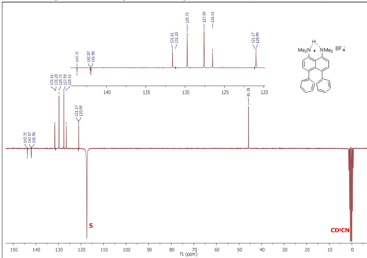
**Fig. S42.**  $^{13}\text{C}\{^1\text{H}\}$  APT-NMR spectrum of compound  $\mathbf{3a}\cdot\text{HBF}_4$  (62.9 MHz, CD<sub>3</sub>CN).
