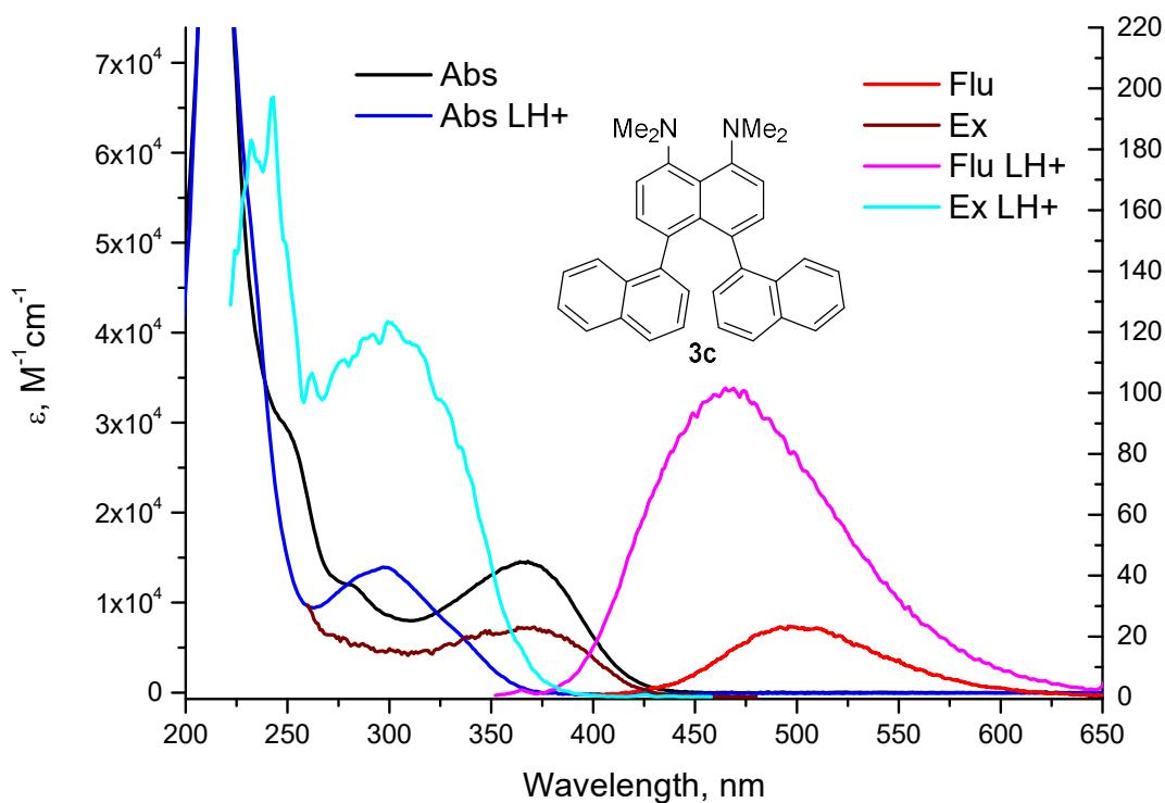
**Fig. S57.** Absorption, excitation, and emission spectra of **3c** (L) and its protonated form **3c-H<sup>+</sup>** (LH<sup>+</sup>) in MeCN, T = 293 K.
