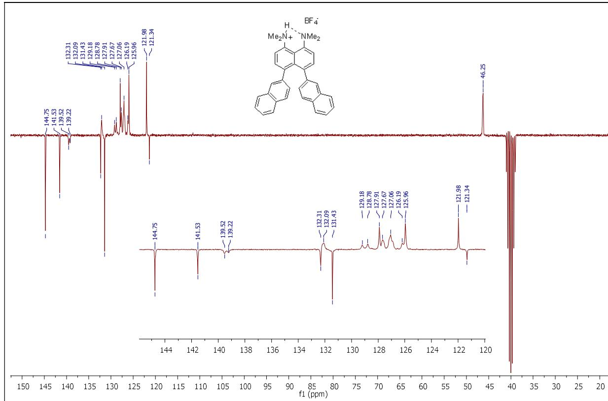
**Fig. S48.**  $^{13}\text{C}\{{}^1\text{H}\}$  APT-NMR spectrum of compound  $3\text{d}\cdot\text{HBF}_4$  (62.9 MHz,  $\text{DMSO-d}_6$ ).
