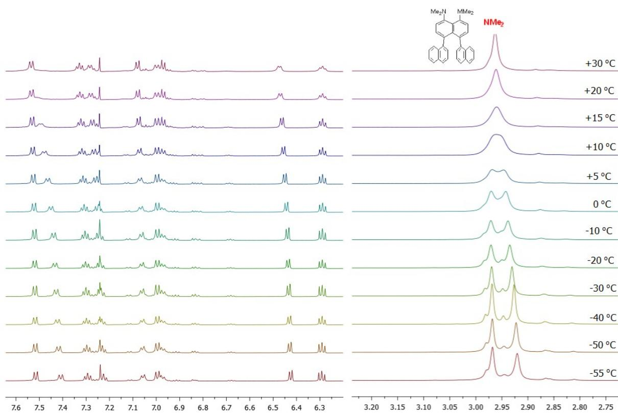
**Fig. S53.** Variable-temperature  $^1\text{H}$  NMR spectra of **3c** ( $\text{CDCl}_3$ , 600 MHz).
