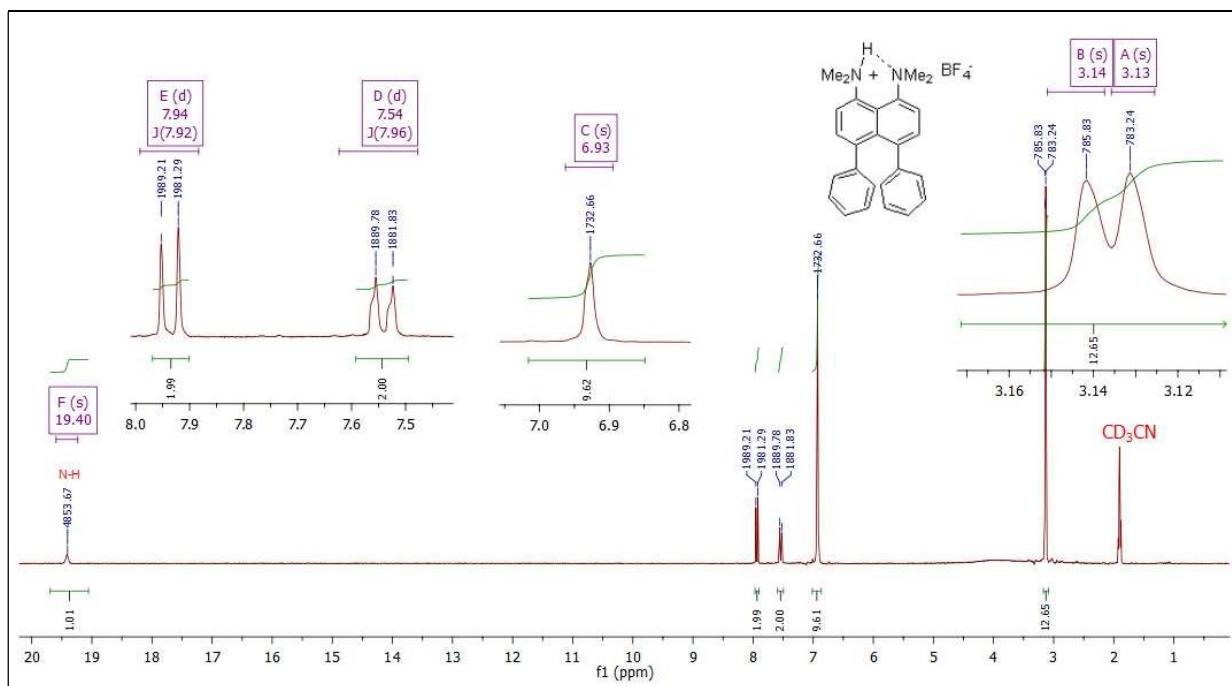
**Fig. S41.**  $^1\text{H}$  NMR spectrum of compound  $\mathbf{3a}\cdot\text{HBF}_4$  (250 MHz, CD<sub>3</sub>CN).
