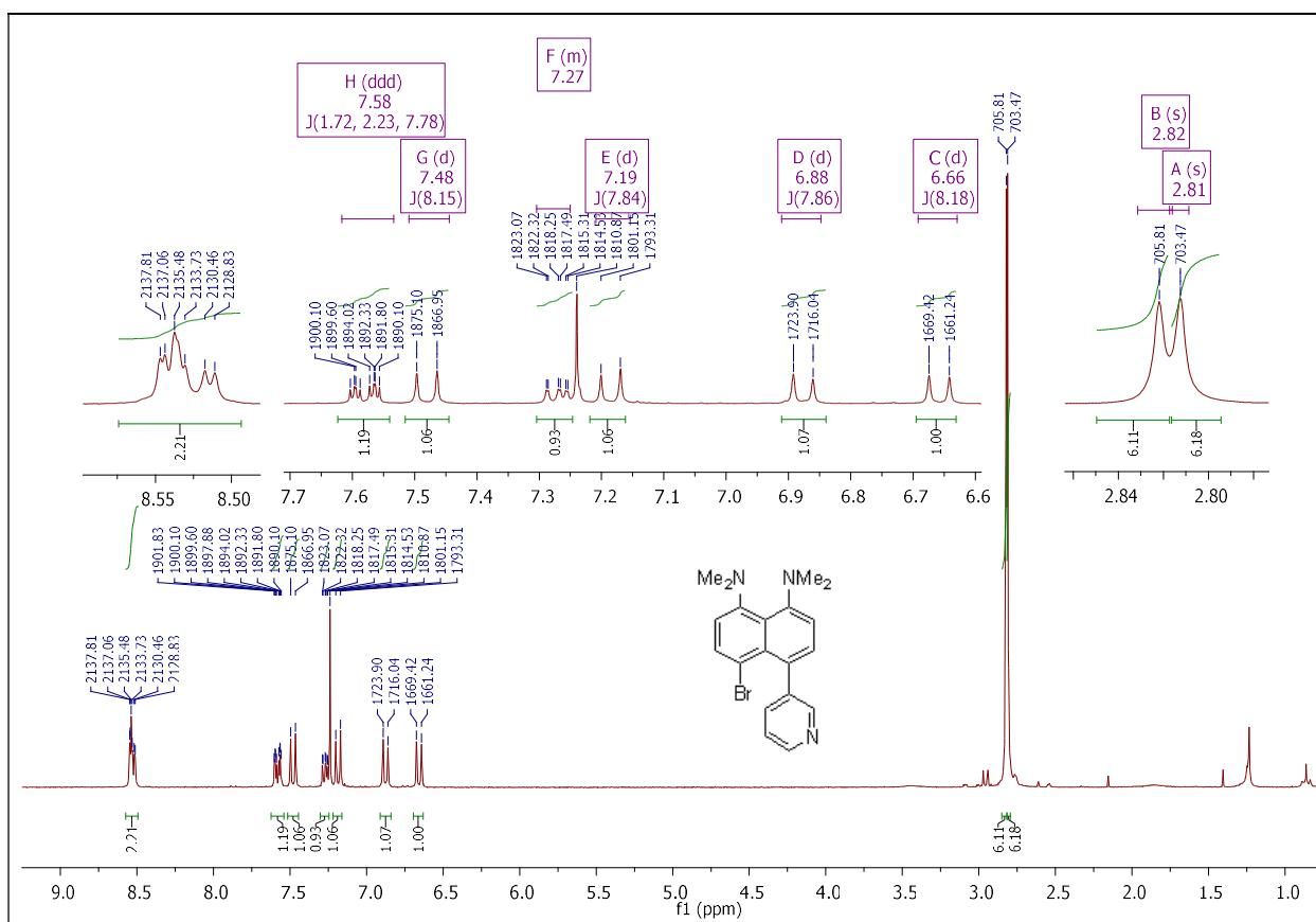
**Fig. S35.**  $^1\text{H}$  NMR spectrum of compound 8 (250 MHz,  $\text{DMSO-d}_6$ ).
