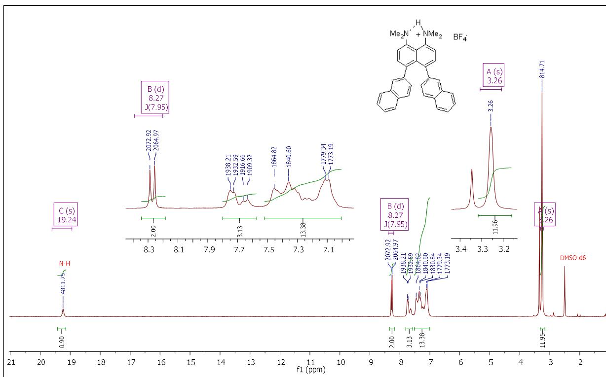
**Fig. S47.**  $^1\text{H}$  NMR spectrum of compound  $3\text{d}\cdot\text{HBF}_4$  (250 MHz,  $\text{DMSO-d}_6$ ).
