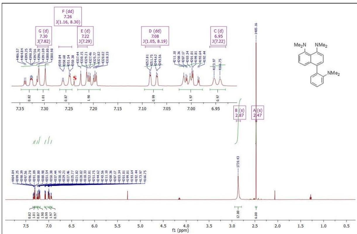
**Fig. S13.**  $^1\text{H}$  NMR spectrum of compound **5g** (600 MHz,  $\text{CDCl}_3$ ).
