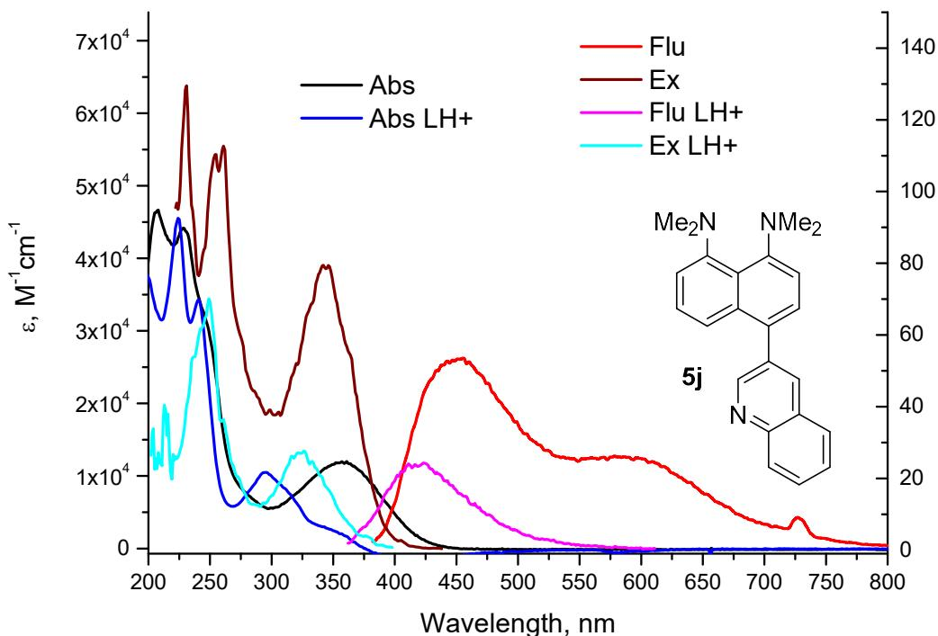
**Fig. S55.** Absorption, excitation, and emission spectra of **5j** (L) and its protonated form **5j-H<sup>+</sup>** (LH<sup>+</sup>) in MeCN, T = 293 K.
