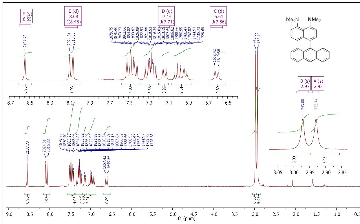
**Fig. S23.**  $^1\text{H}$  NMR spectrum of compound **5l** (250 MHz,  $\text{CDCl}_3$ ).
