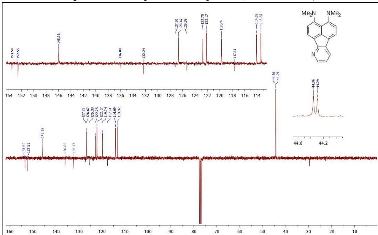
**Fig. S38.**  $^{13}\text{C}\{\text{H}\}$  APT-NMR spectrum of compound 9 (62.9 MHz,  $\text{CDCl}_3$ ).
