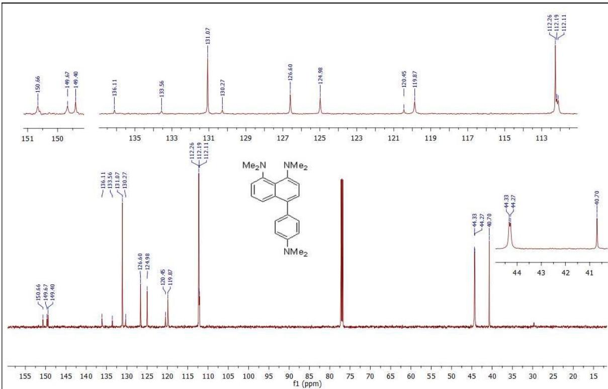
Fig. S12. <sup>13</sup>C{<sup>1</sup>H} NMR spectrum of compound **5f** (150 MHz, CDCl<sub>3</sub>).
