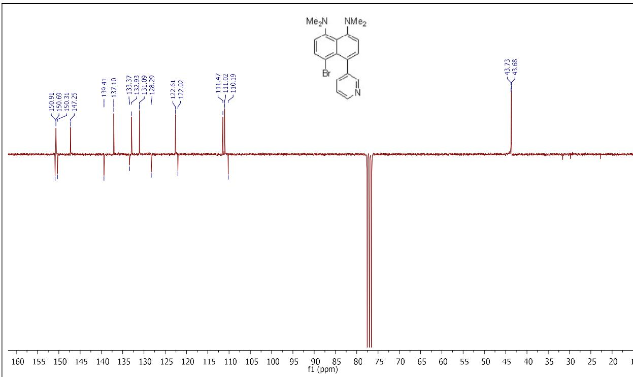
**Fig. S36.**  $^{13}\text{C}\{^1\text{H}\}$  APT-NMR spectrum of compound 8 (62.9 MHz,  $\text{DMSO-d}_6$ ).
