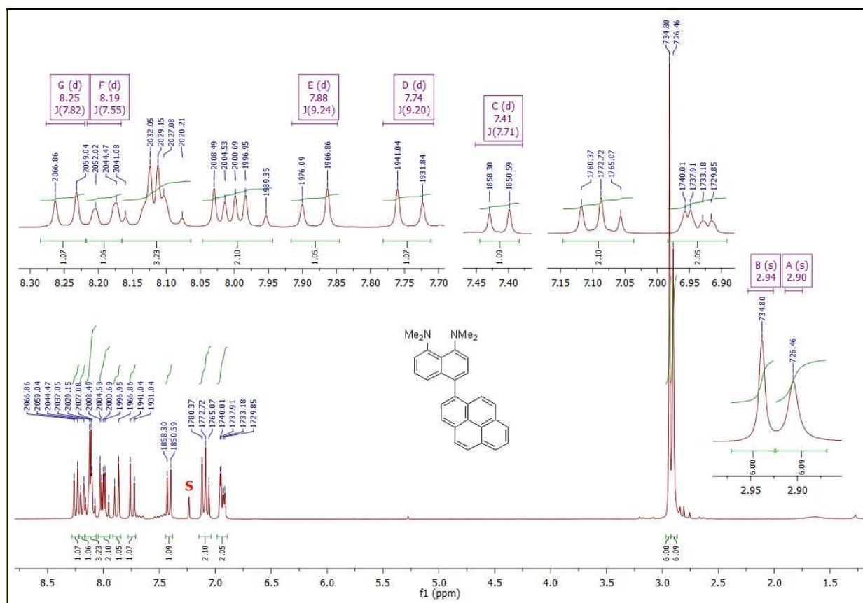
**Fig. S21.**  $^1\text{H}$  NMR spectrum of compound **5k** (250 MHz,  $\text{CDCl}_3$ ).
