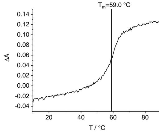
**Figure S9.** Melting profile of **RNA1-RNAG**; 2.5  $\mu$ M RNA, 10 mM Na-Pi buffer, 250 mM NaCl, pH 7, 20  $^{\circ}$ C, 0.7  $^{\circ}$ C/min.
