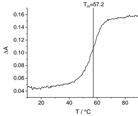
**Figure S15.** Melting profile of **RNA2-RNAG**; 2.5  $\mu\text{M}$  RNA, 10 mM Na-Pi buffer, 250 mM NaCl, pH 7, 20  $^\circ\text{C}$ , 0.7  $^\circ\text{C}/\text{min}$ .
