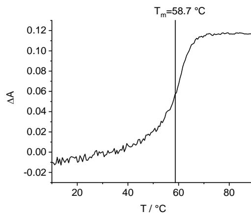
**Figure S11.** Melting profile of **RNA1-RNAS**; 2.5  $\mu$ M RNA, 10 mM Na-Pi buffer, 250 mM NaCl, pH 7, 20  $^{\circ}$ C, 0.7  $^{\circ}$ C/min.
