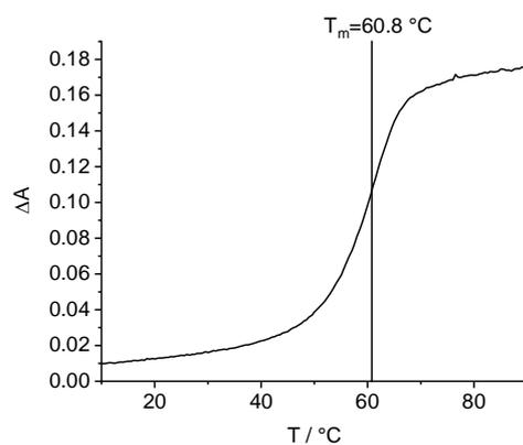
**Figure S7.** Melting profile of **RNA1-RNAA**; 2.5  $\mu\text{M}$  RNA, 10 mM Na-Pi buffer, 250 mM NaCl, pH 7, 20  $^\circ\text{C}$ , 0.7  $^\circ\text{C}/\text{min}$ .
