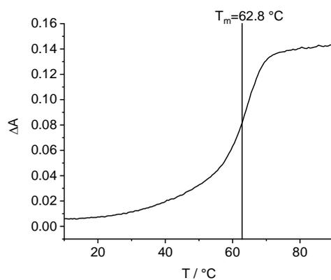
**Figure S6.** Melting profile of **RNA1-RNAD**; 2.5  $\mu\text{M}$  RNA, 10 mM Na-Pi buffer, 250 mM NaCl, pH 7, 20  $^\circ\text{C}$ , 0.7  $^\circ\text{C}/\text{min}$ .
