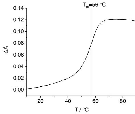
**Figure S12.** Melting profile of **RNA2D**; 2.5  $\mu\text{M}$  RNA, 10 mM Na-Pi buffer, 250 mM NaCl, pH 7, 20  $^\circ\text{C}$ , 0.7  $^\circ\text{C}/\text{min}$ .
