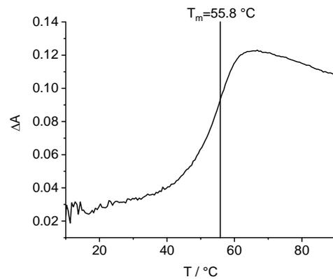
**Figure S17.** Melting profile of **RNA2-RNAS**; 2.5  $\mu\text{M}$  RNA, 10 mM Na-Pi buffer, 250 mM NaCl, pH 7, 20  $^\circ\text{C}$ , 0.7  $^\circ\text{C}/\text{min}$ .
