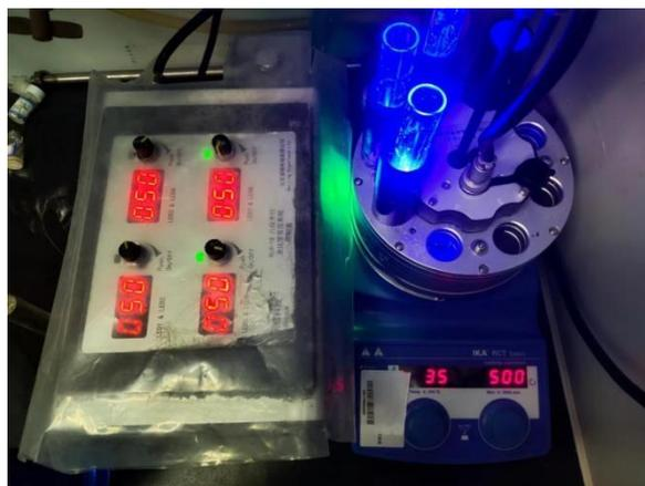
Figure 1. Setup for photocatalytic reactions
