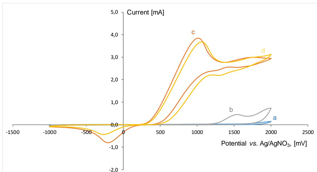
**Figure 1.** CV curve for on a working disc glassy-carbon electrode (d = 3 mm) under a scan rate of 0.1 V/s for (a) background, (b) **1a** (0.05 M), (c) NH<sub>4</sub>SCN (0.25 M), (d) mixture **1a** (0.05 M) with NH<sub>4</sub>SCN (0.25 M) in 0.1 M *n*-Bu<sub>4</sub>NBF<sub>4</sub> in CH<sub>3</sub>CN/HCOOH (8/2).
