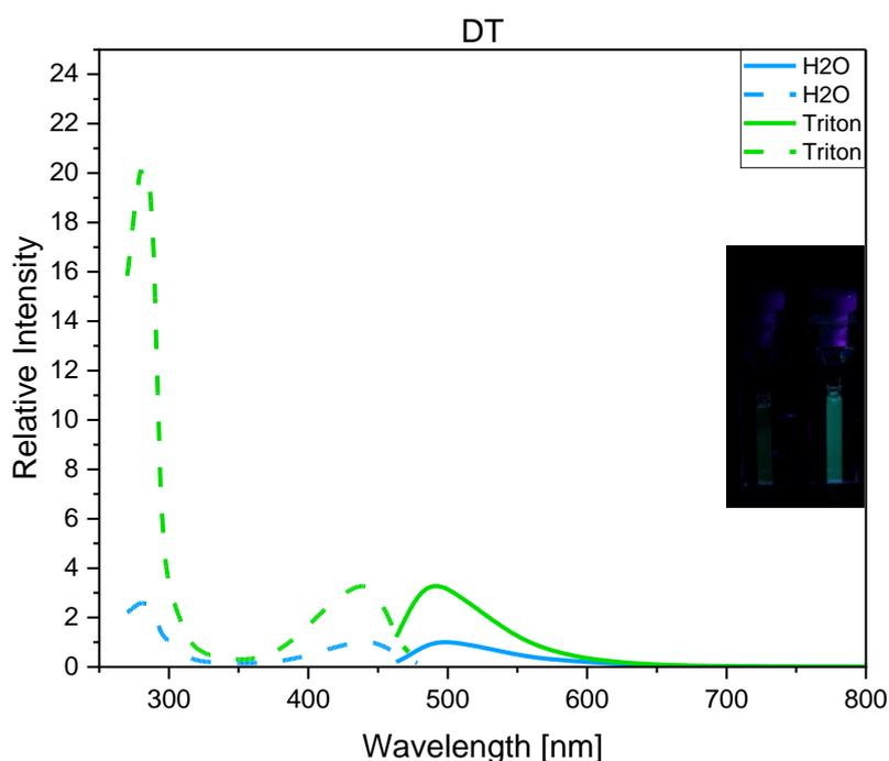
**Figure S35:** Emission enhancement of **DT** in water and in aqueous solution of Triton X-100 (compound conc. = 10  $\mu\text{M}$ , Triton X-100 conc. = 500  $\mu\text{M}$ ). Emission maximum of **DT** in water was set to 1. Picture shows **DT** in water without (left) and with Triton-X 100 (right), irradiated with 395 nm.
