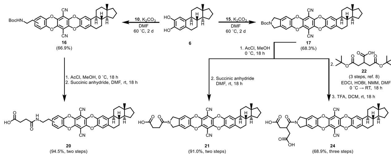
**Figure S4:** Synthesis of carboxylic acids **20–24**. Compound **22**<sup>8</sup> was synthesized according to the respective literature protocol.
