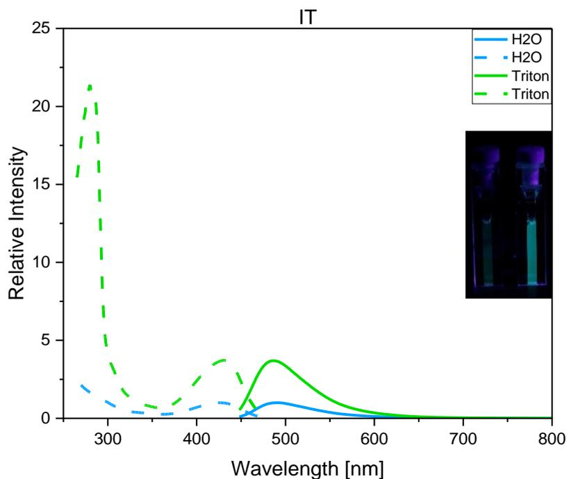
**Figure S36:** Emission enhancement of **IT** in water and in aqueous solution of Triton X-100 (compound conc. = 10  $\mu$ M, Triton X-100 conc. = 500  $\mu$ M). Emission maximum of **IT** in water was set to 1. Picture shows **IT** in water without (left) and with Triton-X 100 (right), irradiated with 395 nm.
