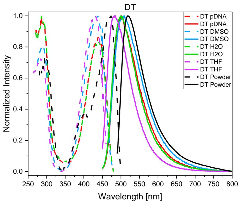
**Figure S32:** Normalized luminescence spectra of **DT** (dotted line: excitation; solid line: emission; conc. = 10  $\mu$ M, conc. pDNA = 500 ng/mL).
