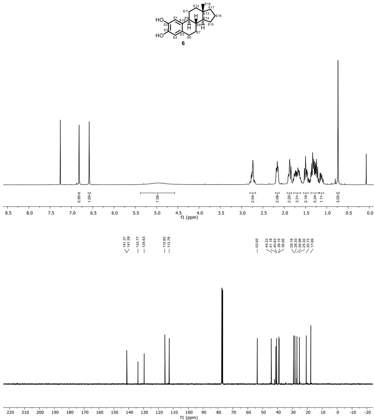
**Figure S7:** <sup>1</sup>H- (top, 400 MHz, CDCl<sub>3</sub>, 298 K) and <sup>13</sup>C-NMR spectrum (bottom, 101 MHz, CDCl<sub>3</sub>, 298 K) of compound 6.
