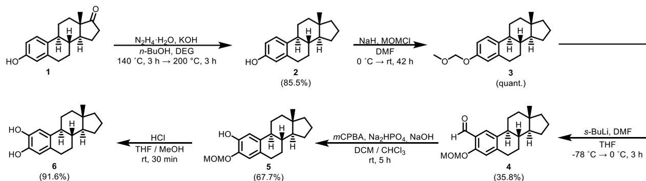
**Figure S1:** Synthesis of estrone catechol precursor **6**. Compounds **2**<sup>4</sup> and **3–5**<sup>5</sup> were synthesized according to modified literature protocols.
