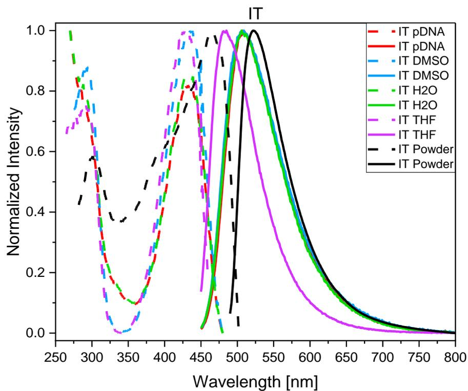
**Figure S33:** Normalized luminescence spectra of IT (dotted line: excitation; solid line: emission; conc. = 10  $\mu$ M, conc. pDNA = 500 ng/mL).
