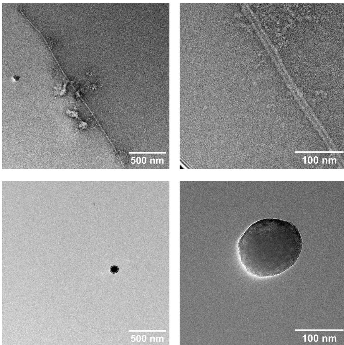
**Figure S30:** TEM images (left: overview; right: zoom) of ligand IT<sub>2</sub> (10  $\mu$ M) in water (top) and in the presence of pDNA (bottom, 500 ng/mL).
