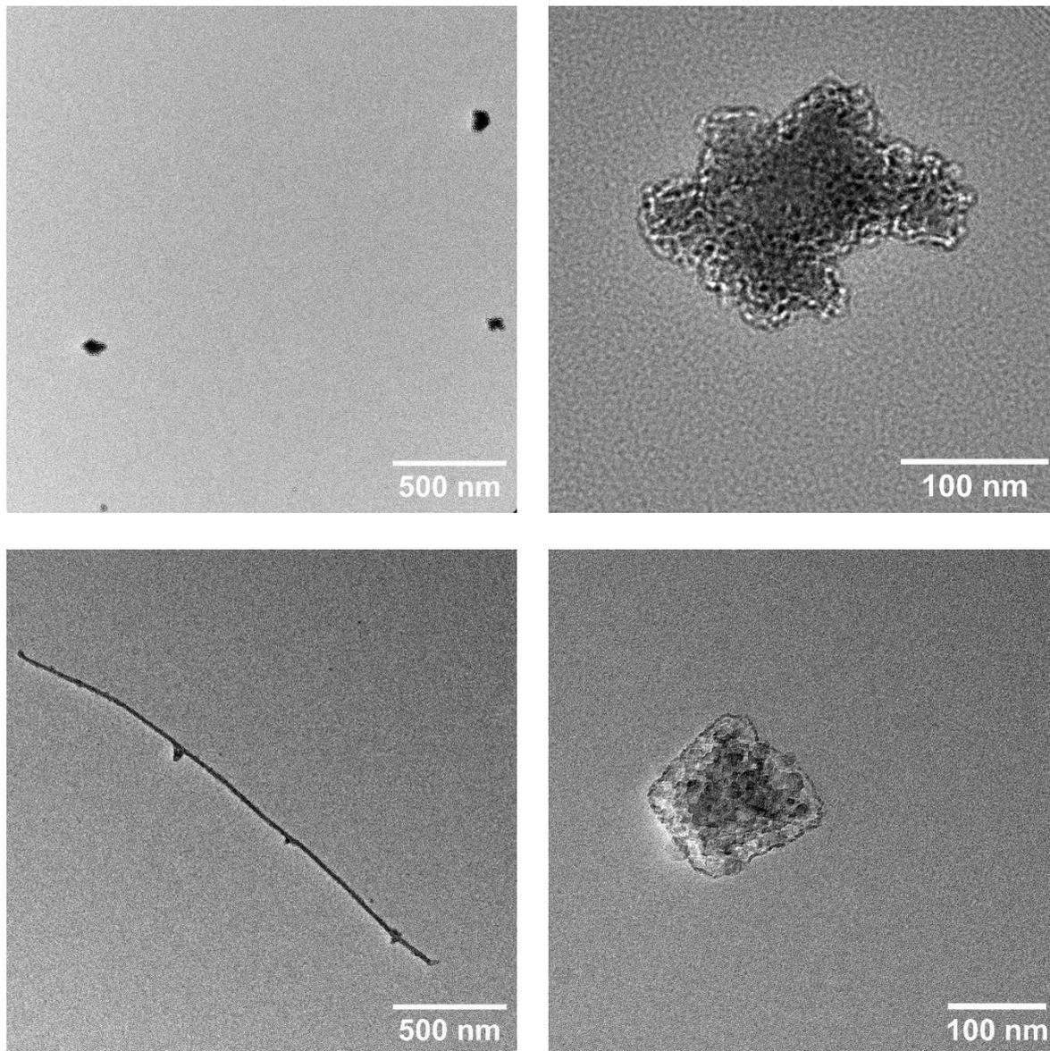
**Figure S29:** TEM images (left: overview; right: zoom) of ligand **IT** (10  $\mu$ M) in water (top) and in the presence of pDNA (bottom, 500 ng/mL). The lower left picture showing rods in the presence of pDNA indicates uncomplete lipoplex formation.
