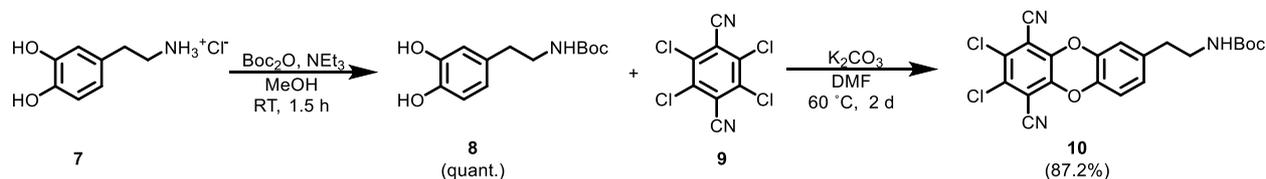
**Figure S2:** Synthesis of dopamine precursor **10**. Compound **8**<sup>6</sup> was synthesized according to a modified literature protocol.
