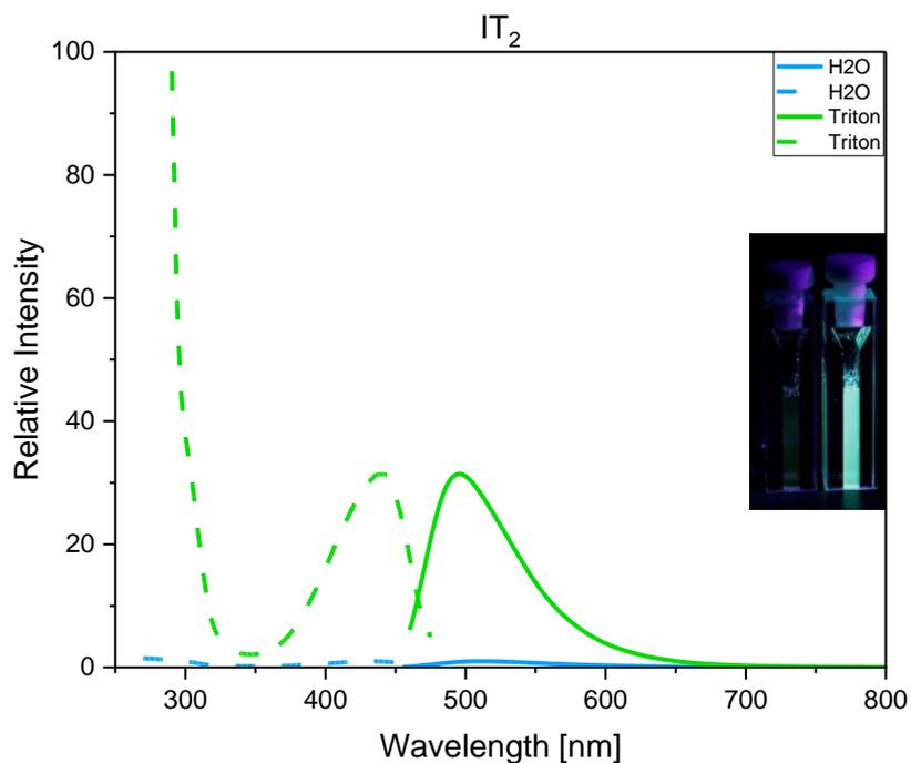
**Figure S37:** Emission enhancement of **IT<sub>2</sub>** in water and in aqueous solution of Triton X-100 (compound conc. = 10  $\mu$ M, Triton X-100 conc. = 500  $\mu$ M). Emission maximum of **IT<sub>2</sub>** in water was set to 1. Picture shows **IT<sub>2</sub>** in water without (left) and with Triton-X 100 (right), irradiated with 395 nm.
