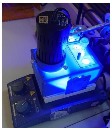
Figure S1. Irradiation setup, EvoluChem™ PhotoRedOx Box, 450 nm / 30 W blue LED.
