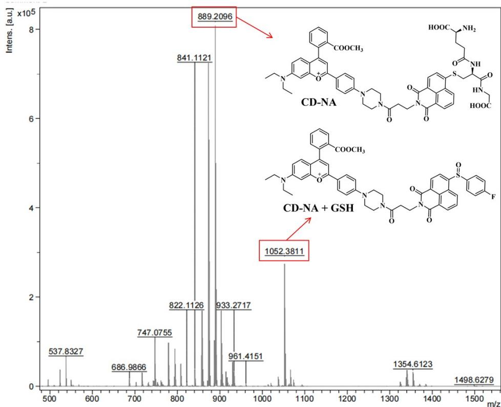
**Figure S6.** The mass spectrum of CD-NA in the presence of GSH.
