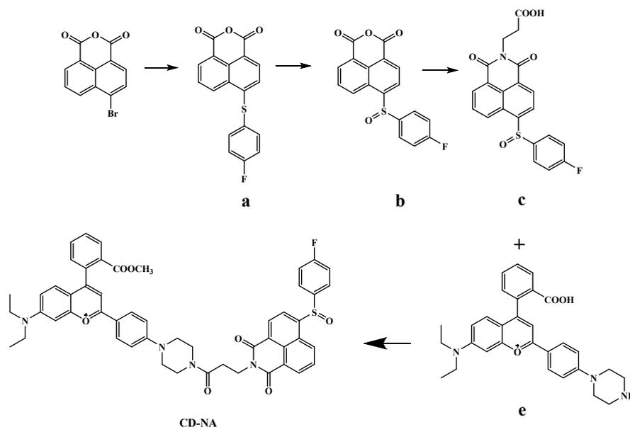
**Figure S1.** The synthetic procedures of CD-NA.
