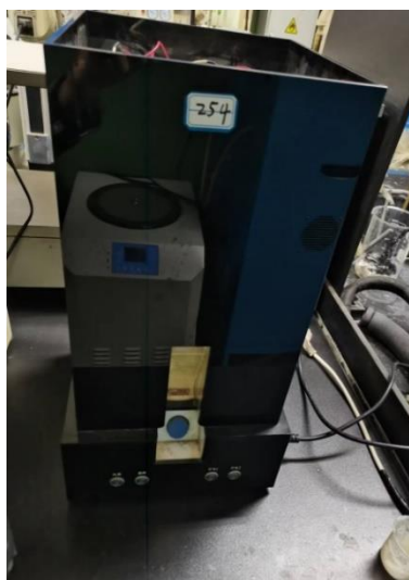
Figure S2. 254 nm ultraviolet lamp (64 W)
