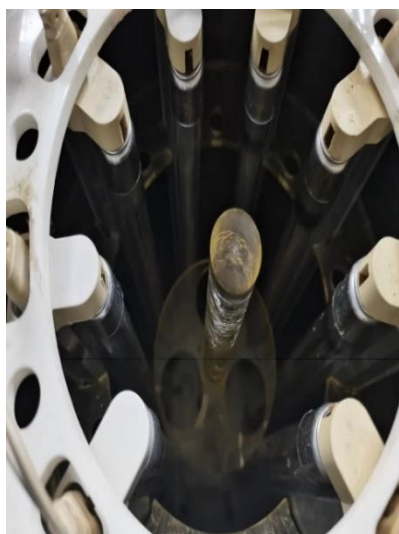
Figure S2. 254 nm ultraviolet lamp (64 W)
