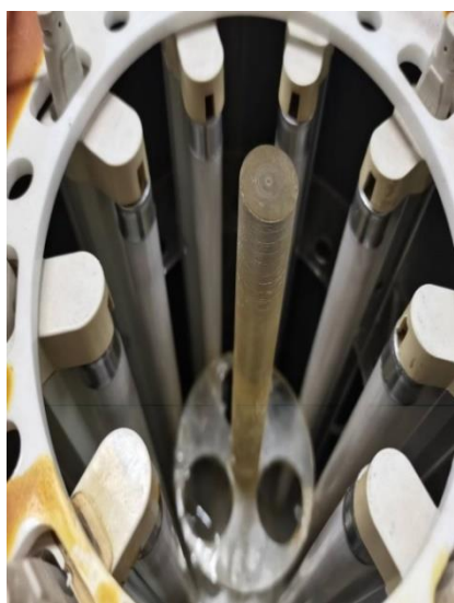
Figure S1. 313 nm ultraviolet lamp (64 W)
