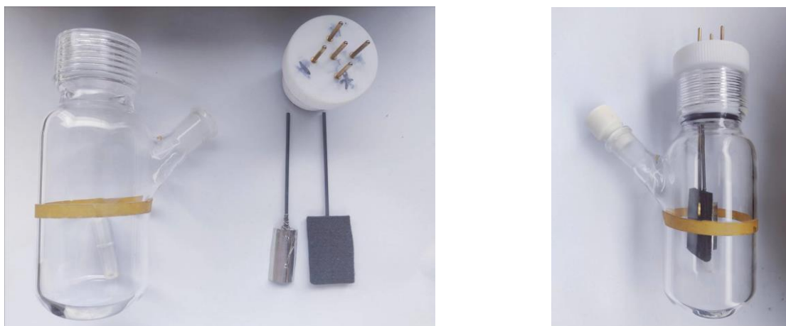
Figure S2. Components of the reaction setup (left). Assembled reaction vessel (right).
