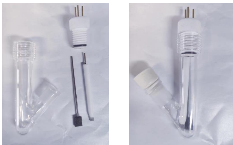
Figure S1. Components of the reaction setup (left). Assembled reaction vessel (right)
