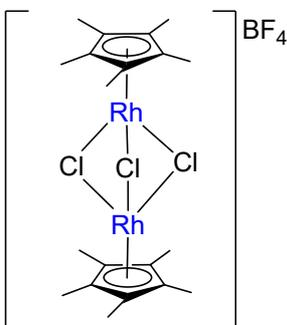
**Rh-III-1** (100 mg, 0.16 mmol, 1 equiv), 2M  $\text{HBF}_4$  (0.2 ml, 0.4 mmol, 2.5 equiv), and MeOH (2 mL) were placed in a Schlenk tube and were refluxed for 5 minutes. The reaction mixture was then kept at  $4^\circ\text{C}$  for 8 hours. The formed crystals were centrifuged off, crushed, washed with MeOH (5 ml) and dried in vacuo. The yield of **Rh-III-3** is 84 mg (79%).
