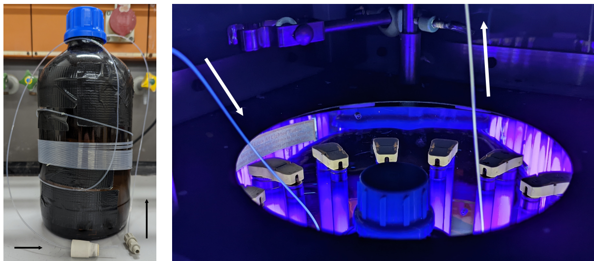
Figure S1. Flow reactor (left) and flow reactor inside the Rayonet reactor (right).
