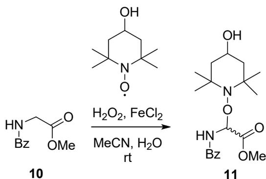
**TEMPOL-glycine adduct**: A solution of *N*-benzoyl glycine methyl ester (**10**, 163 mg, 0.85 mmol), TEMPOL (120 mg, 0.696 mmol) and FeCl<sub>2</sub> (10 mg, 0.085 mmol) in 1:1 H<sub>2</sub>O: MeCN
