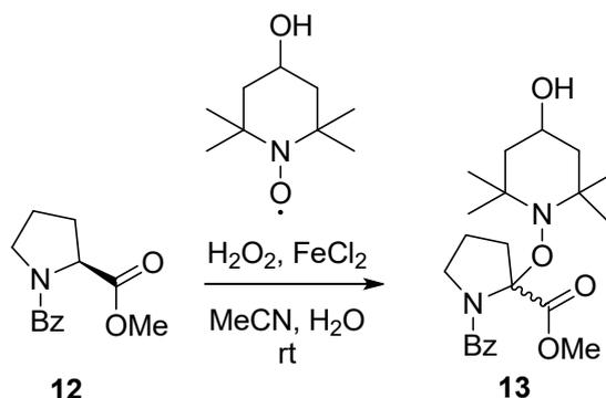
**TEMPOL-proline adduct:** A solution of benzoyl protected proline methyl ester (**12**, 172 mg, 0.748 mmol), TEMPOL (108 mg, 0.627 mmol) and FeCl<sub>2</sub> (9.5 mg, 0.0748 mmol) in 1:1 H<sub>2</sub>O:MeCN (7 mL) was stirred under N<sub>2</sub> atmosphere for 3 h. The crude mixture was concentrated *in vacuo* to a crude product of **13**.
