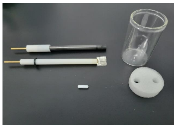
Figure S1. The materials used to make the electrolytic cell for the synthesis of 3-
