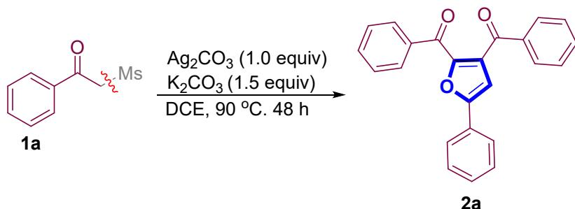
A 75 mL Schlenk tube was charged with 2-(methylsulfonyl)-1-phenylethan-1-one **1a** (10 mmol),  $\text{Ag}_2\text{CO}_3$  (10 mmol),  $\text{K}_2\text{CO}_3$  (15 mmol) and DCE (30 mL). The reaction mixture was stirred for 48 hours at 90 °C (oil bath). After that it was filtered through a short pad of Celite® and washed with ethyl acetate. The solvent was then evaporated under reduced pressure and the crude was purified by column chromatography on silica gel to afford the pure product **2a**.
