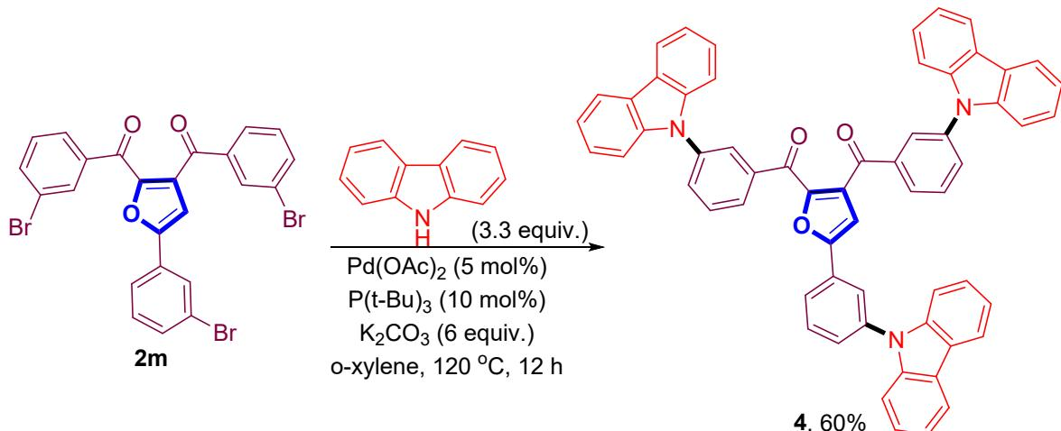
**2m** (0.2 mmol), Pd(OAc)<sub>2</sub> (5 mol%), P(t-Bu)<sub>3</sub> (10 mol%), K<sub>2</sub>CO<sub>3</sub> (1.2 mmol) and 9H-carbazole (0.66 mmol) were dissolved in o-xylene (2 ml) under Ar atmosphere, then the mixture was stirred at 120 °C for 12 hour. The solvent was removed in vacuo and the residue was chromatographed on silica gel (petroleum ether:diethyl ether 5:1) to yield in **4** (60% yield)
