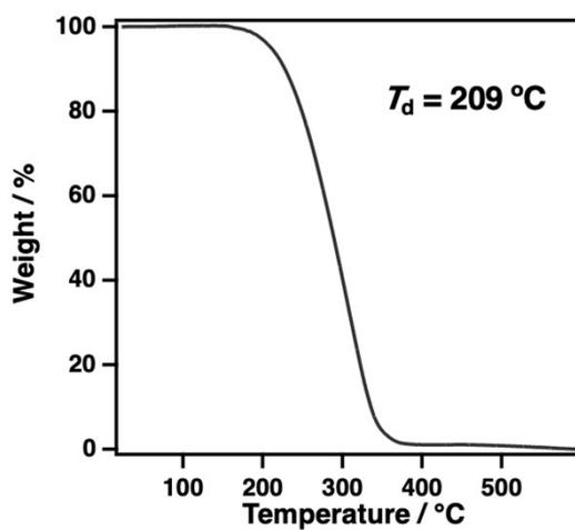
Figure S2. TGA trace of DBM.
