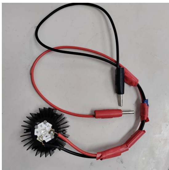
Figure S 1 The image of LED (ILA-HSINK-STAR-50*20 mm) used in the photo flow experiments.
