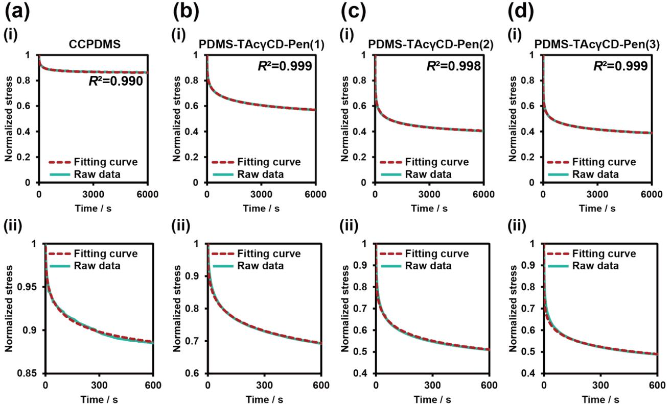
**Fig. S13.** Stress relaxation curves of (a) CCPDMS and (f) PDMS-TAc $\gamma$ CD-Pen( $x$ ) when  $x =$  (b) 1, (b) 2, and (b) 3 with fitting curves over the entire range (6000 seconds). The parameters for fitting curves were determined from the entire range and fixed when focused on the range by 600 seconds (i) Plots by 6000 seconds and (ii) plots by 600 seconds (raw data: cyan solid line, fitting curves: red dashed line).
