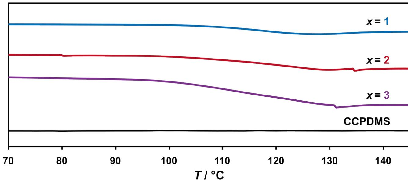
**Fig. S15.** Zoomed DSC thermograms of CCPDMS, PDMS-TAc $\gamma$ CD-Pen(1), PDMS-TAc $\gamma$ CD-Pen(2), and PDMS-TAc $\gamma$ CD-Pen(3) on the second scan.
