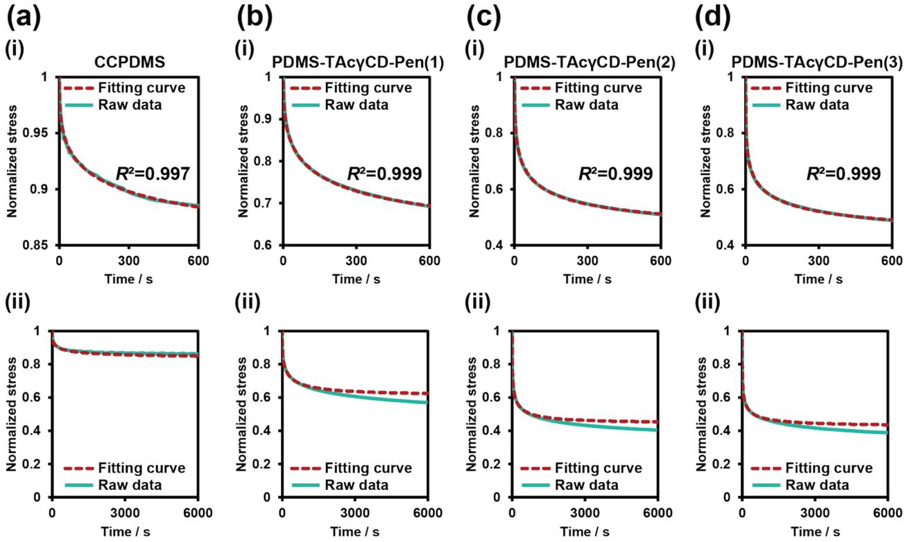
**Fig. S12.** Stress relaxation curves of (a) CCPDMS and (f) PDMS-TAc $\gamma$ CD-Pen( $x$ ) when  $x =$  (b) 1, (b) 2, and (b) 3 with fitting curves focusing on the initial 600 second regime. The parameters for fitting curves were determined from the 600 second regime and fixed when expanded the range by 6000 seconds. (i) Plots by 600 seconds and (ii) plots by 6000 seconds (raw data: cyan solid line, fitting curves: red dashed line).
