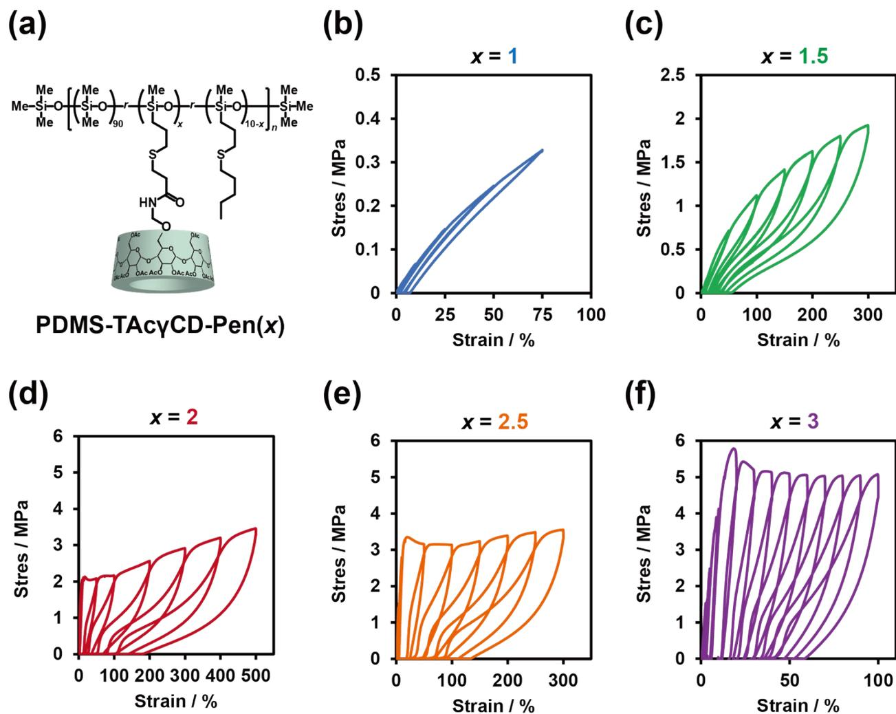
**Fig. S11.** (a) Chemical structure of PDMS-TAc $\gamma$ CD-Pen( $x$ ) and cyclic stress–strain curves of PDMS-TAc $\gamma$ CD-Pen( $x$ ) when  $x =$  (b) 1, (c) 1.5, (d) 2, (e) 2.5, and (f) 3.
