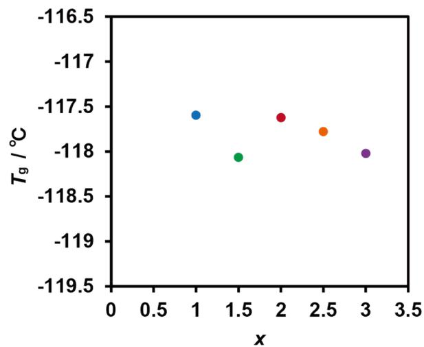
**Fig. S14.** (a) DSC thermograms of CCPDMS and PDMS-TAc $\gamma$ CD-Pen( $x$ ) on the second scan and (b)  $T_g$  versus the amount of TAc $\gamma$ CD ( $x = 1, 1.5, 2, 2.5,$  and  $3$ ).
