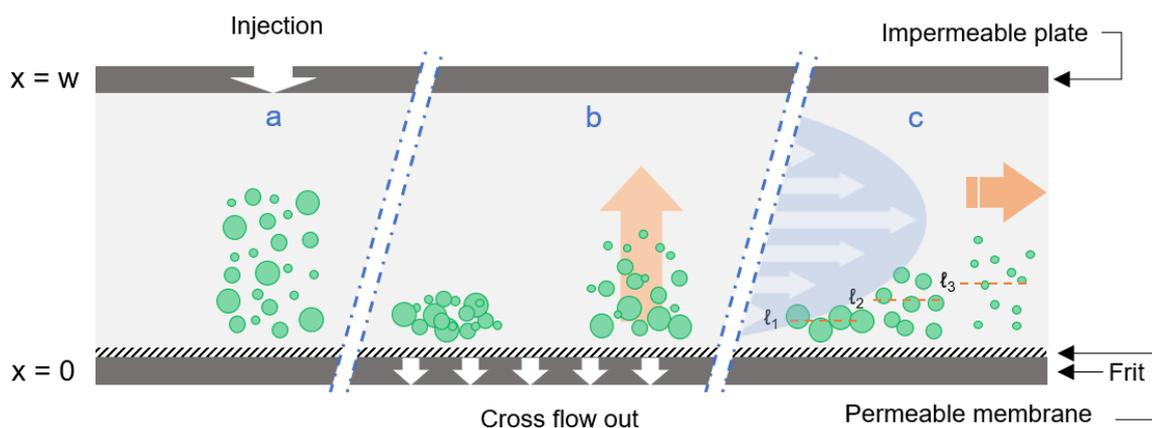
**Figure SI17:** Simplified scheme of an AF4 channel operating in the normal mode. It depicts a) sample injection, b) sample focusing, and c) separation of the particle "clouds" with mean layer thickness  $l_n$ .
