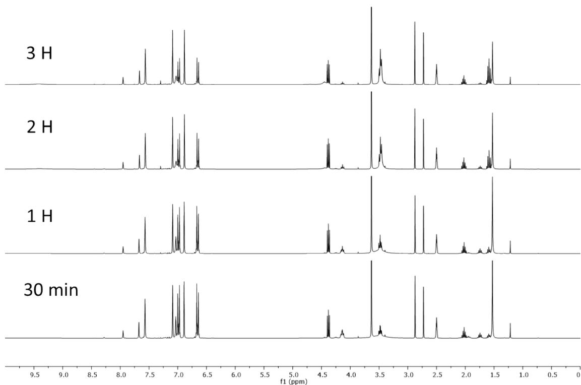
**Figure S18.** Kinetics of the depolymerisation of BPA-PC monitored through  $^1\text{H}$  NMR spectroscopy carried out with 1 eq. of imidazole as catalyst, 1.05 eq. of 1,3-propanediol as nucleophile and 2.5 eq. of 1-Methylimidazole as solvent, after 3 h at 50 °C.
