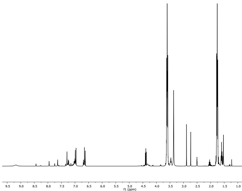
**Figure S4.** <sup>1</sup>H NMR spectra of the crude product of the depolymerisation of BPA-PC carried out with 1 eq. of imidazole as catalyst, 1.05 eq. of 1,3-propanediol as nucleophile and 10 eq. of THF as solvent, after 3 h at 50 °C.
