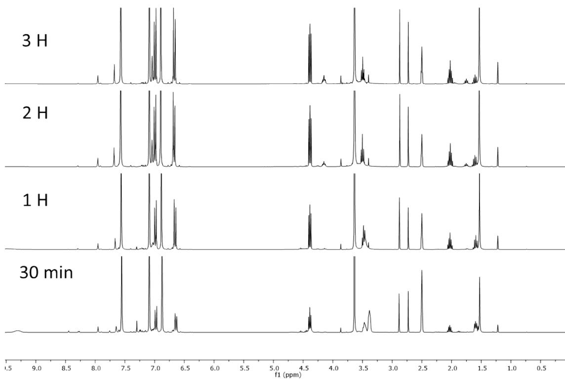
**Figure S16.** Kinetics of the depolymerisation of BPA-PC monitored through  $^1\text{H}$  NMR spectroscopy carried out with 1 eq. of imidazole as catalyst, 1.5 eq. of 1,3-propanediol as nucleophile and 10 eq. of 1-Methylimidazole as solvent, after 3 h at 50 °C.
