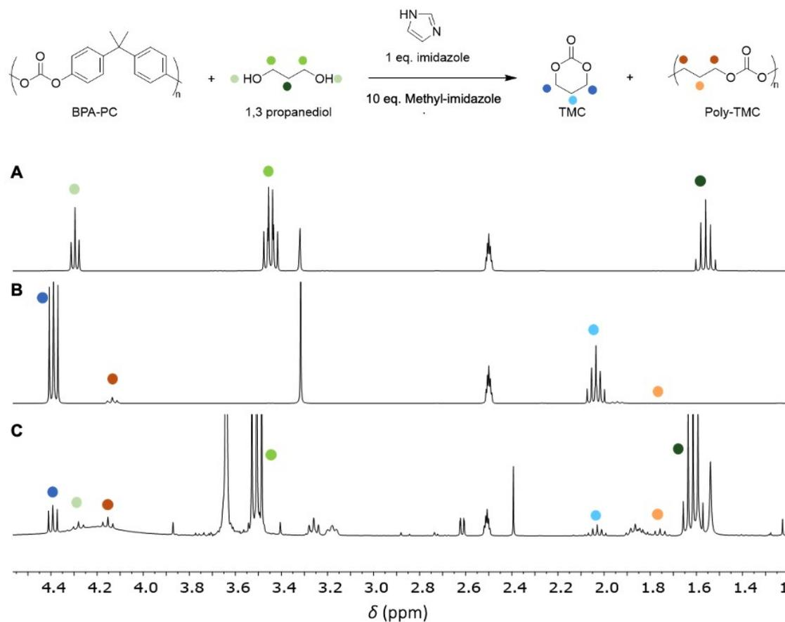
**Figure S1.**  $^1\text{H}$  NMR spectra and assignment of **A.** the reactant, 1,3-propanediol, **B.** the products formed, TMC and PTMC, and **C.** the crude of the depolymerisation reaction.
