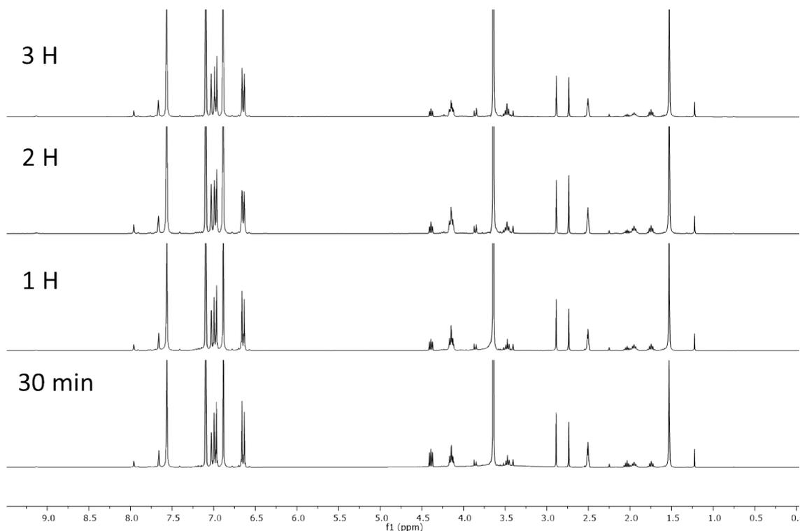
**Figure S14.** Kinetics of the depolymerisation of BPA-PC monitored through  $^1\text{H}$  NMR spectroscopy carried out with 1 eq. of imidazole as catalyst, 1.05 eq. of 1,3-propanediol as nucleophile and 10 eq. of 1-Methylimidazole as solvent, after 3 h at 90 °C.
