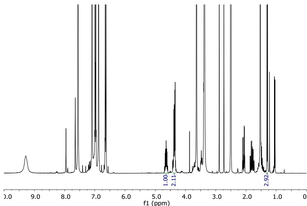
**Figure S26.**  $^1\text{H}$  NMR spectrum of the crude product of the depolymerisation of BPA-PC carried out with 1 eq. of imidazole as catalyst, 1.05 eq. of 1,3-butanediol as nucleophile and 10 eq. of 1-methylimidazole as solvent, after 3 h at 50 °C.
