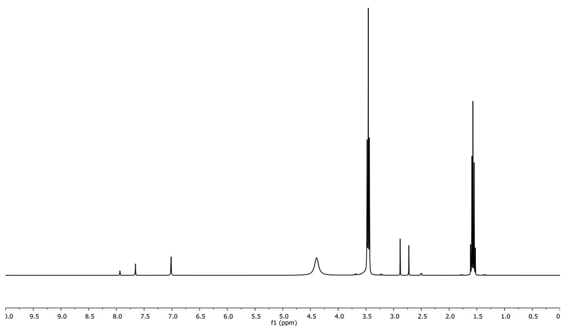
**Figure S2.**  $^1\text{H}$  NMR spectra of the crude product of the depolymerisation of BPA-PC carried out with 1 eq. of imidazole as catalyst, 10 eq. of 1,3-propanediol as nucleophile, in bulk, after 3 h at 50 °C. No conversion was observed.
