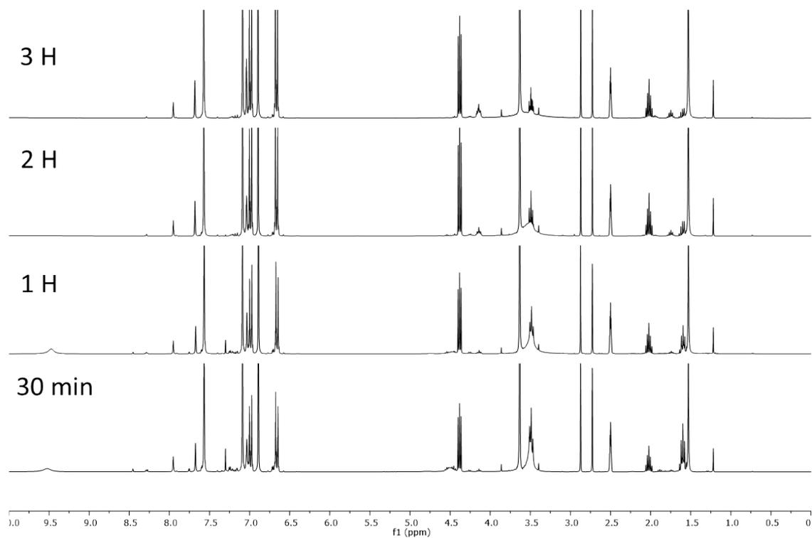
**Figure S19.** Kinetics of the depolymerisation of BPA-PC monitored through  $^1\text{H}$  NMR spectroscopy carried out with 1 eq. of imidazole as catalyst, 1.05 eq. of 1,3-propanediol as nucleophile and 5 eq. of 1-Methylimidazole as solvent, after 3 h at 50 °C.
