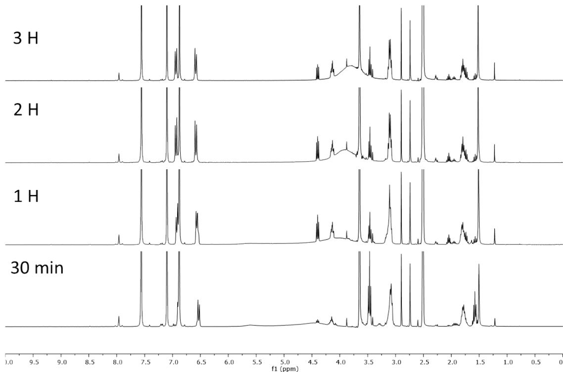
**Figure S11.** Kinetics of the depolymerisation of BPA-PC monitored through  $^1\text{H}$  NMR spectroscopy carried out with 1 eq. of TBD as catalyst, 1.05 eq. of 1,3-propanediol as nucleophile and 10 eq. of 1-Methylimidazole as solvent, after 3 h at 50 °C.
