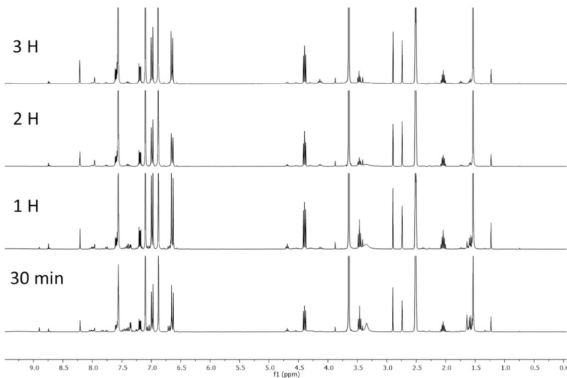
**Figure S8.** Kinetics of the depolymerisation of BPA-PC monitored through <sup>1</sup>H NMR spectroscopy carried out with 1 eq. of benzimidazole as catalyst, 1.05 eq. of 1,3-propanediol as nucleophile and 10 eq. of 1-Methylimidazole as solvent, after 3 h at 50 °C.
