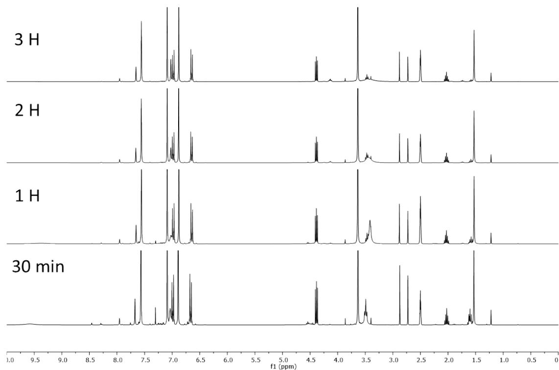
**Figure S23.** Kinetics of the depolymerisation of BPA-PC monitored through <sup>1</sup>H NMR spectroscopy carried out with 2 eq. of imidazole as catalyst, 1.05 eq. of 1,3-propanediol as nucleophile and 10 eq. of 1-Methylimidazole as solvent, after 3 h at 50 °C.
