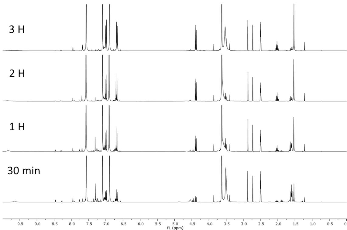
**Figure S20.** Kinetics of the depolymerisation of BPA-PC monitored through <sup>1</sup>H NMR spectroscopy carried out with 1 eq. of imidazole as catalyst, 1.05 eq. of 1,3-propanediol as nucleophile and 20 eq. of 1-Methylimidazole as solvent, after 3 h at 50 °C.
