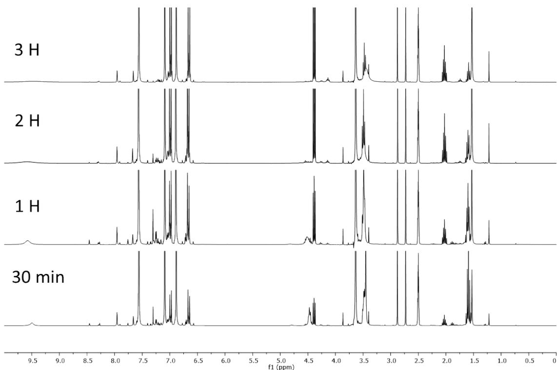
**Figure S22.** Kinetics of the depolymerisation of BPA-PC monitored through <sup>1</sup>H NMR spectroscopy carried out with 0.5 eq. of imidazole as catalyst, 1.05 eq. of 1,3-propanediol as nucleophile and 10 eq. of 1-Methylimidazole as solvent, after 3 h at 50 °C.
