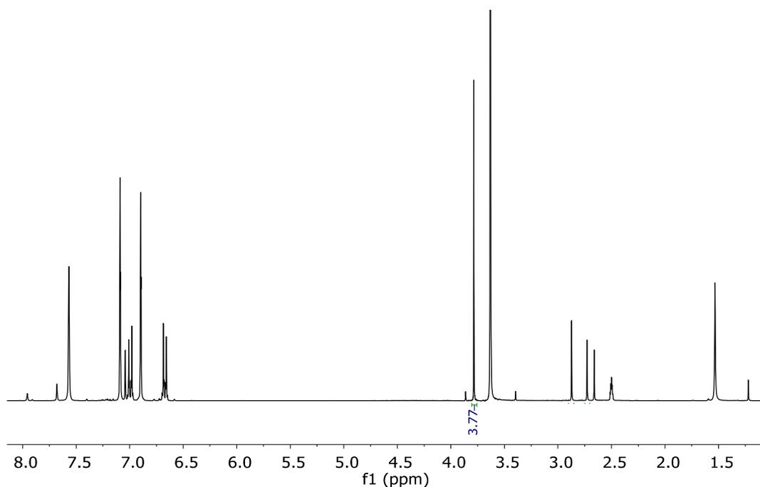
**Figure S29.**  $^1\text{H}$  NMR spectrum of the crude product of the depolymerisation of BPA-PC carried out with 1 eq. of imidazole as catalyst, 1.05 eq. of ethanedithiol as nucleophile and 10 eq. of 1-methylimidazole as solvent, after 3 h at 50 °C.
