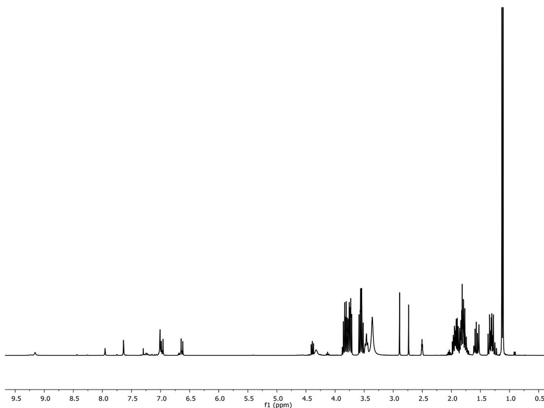
**Figure S6.** <sup>1</sup>H NMR spectra of the crude product of the depolymerisation of BPA-PC carried out with 1 eq. of imidazole as catalyst, 1.05 eq. of 1,3-propanediol as nucleophile and 10 eq. of 2-Methyl-THF as solvent, after 3 h at 50 °C.
