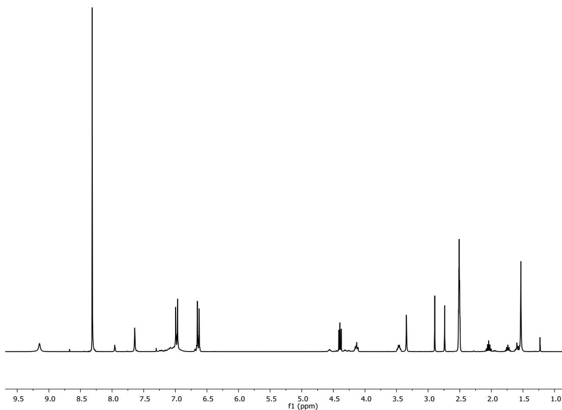
**Figure S5.** <sup>1</sup>H NMR spectra of the crude product of the depolymerisation of BPA-PC carried out with 1 eq. of imidazole as catalyst, 1 eq. of 1,3-propanediol as nucleophile and 10 eq. of chloroform as solvent, after 3 h at 50 °C.
