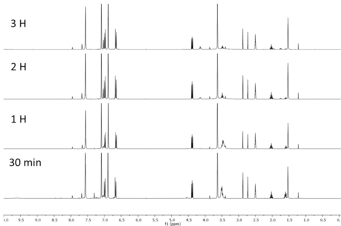
**Figure S13.** Kinetics of the depolymerisation of BPA-PC monitored through  $^1\text{H}$  NMR spectroscopy carried out with 1 eq. of imidazole as catalyst, 1.05 eq. of 1,3-propanediol as nucleophile and 10 eq. of 1-Methylimidazole as solvent, after 3 h at 60 °C.
