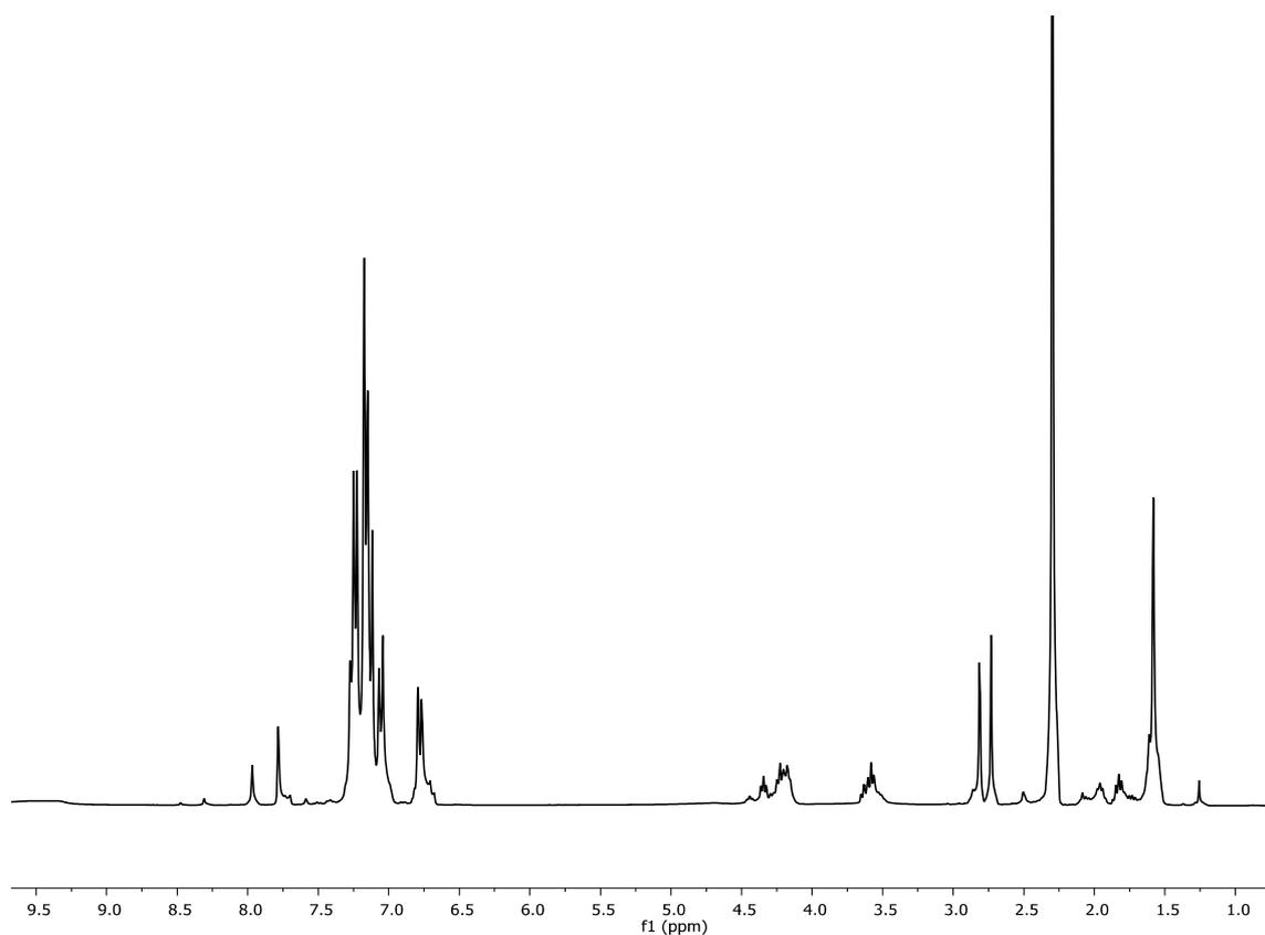
**Figure S7.** <sup>1</sup>H NMR spectra of the crude product of the depolymerisation of BPA-PC carried out with 1 eq. of imidazole as catalyst, 1.05 eq. of 1,3-propanediol as nucleophile and 10 eq. of toluene as solvent, after 3 h at 50 °C.
