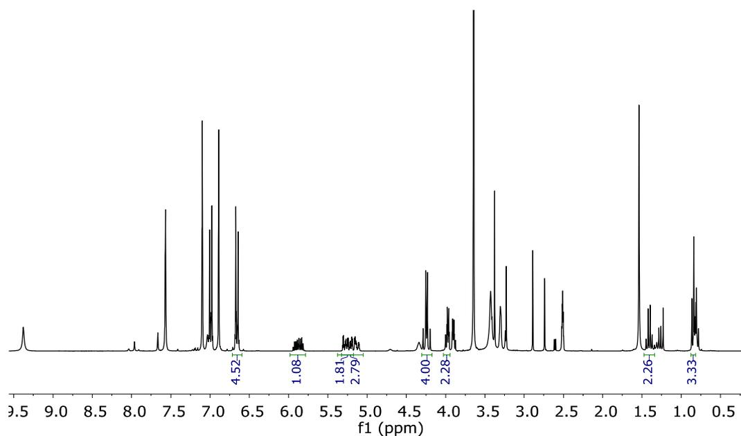
**Figure S28.**  $^1\text{H}$  NMR spectrum of the crude product of the depolymerisation of BPA-PC carried out with 1 eq. of imidazole as catalyst, 1.05 eq. of trimethylolpropane allyl ether as nucleophile and 10 eq. of 1-methylimidazole as solvent, after 3 h at 50 °C.
