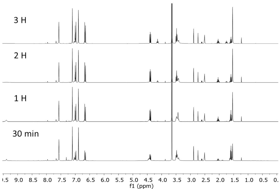
**Figure S17.** Kinetics of the depolymerisation of BPA-PC monitored through  $^1\text{H}$  NMR spectroscopy carried out with 1 eq. of imidazole as catalyst, 1.75 eq. of 1,3-propanediol as nucleophile and 10 eq. of 1-Methylimidazole as solvent, after 3 h at 50 °C.
