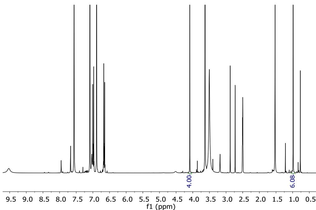
**Figure S27.**  $^1\text{H}$  NMR spectrum of the crude product of the depolymerisation of BPA-PC carried out with 1 eq. of imidazole as catalyst, 1.05 eq. of 2,2-dimethyl propanediol as nucleophile and 10 eq. of 1-methylimidazole as solvent, after 3 h at 50 °C.
