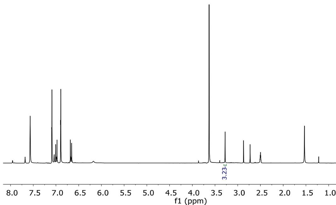
**Figure S30.**  $^1\text{H NMR}$  spectrum of the crude product of the depolymerisation of BPA-PC carried out with 1 eq. of imidazole as catalyst, 1.05 eq. of ethylenediamine as nucleophile and 10 eq. of 1-methylimidazole as solvent, after 3 h at 50 °C.
