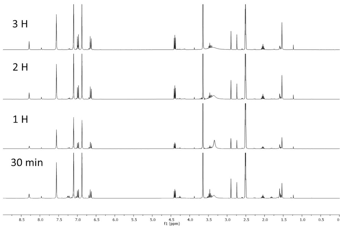
**Figure S9.** Kinetics of the depolymerisation of BPA-PC monitored through <sup>1</sup>H NMR spectroscopy carried out with 1 eq. of triazole as catalyst, 1.05 eq. of 1,3-propanediol as nucleophile and 10 eq. of 1-Methylimidazole as solvent, after 3 h at 50 °C.
