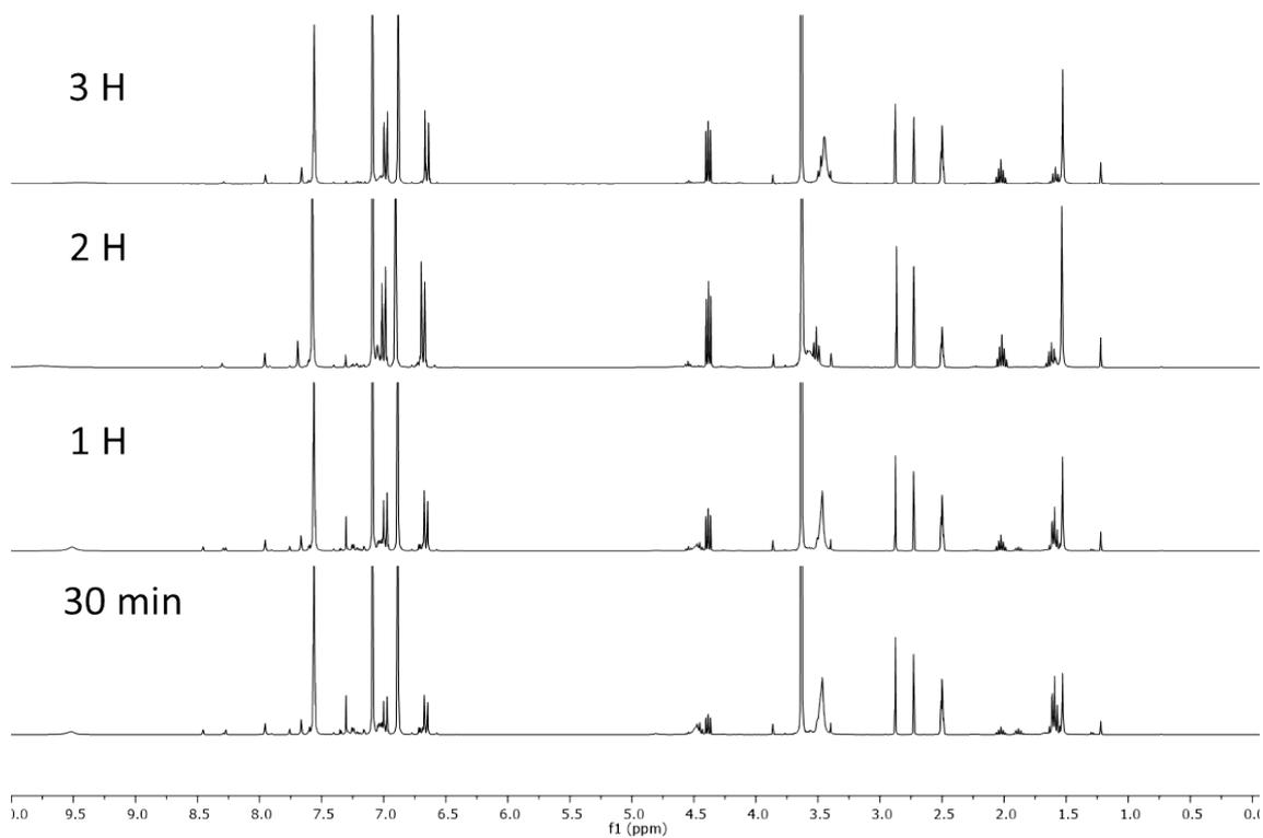
**Figure S12.** Kinetics of the depolymerisation of BPA-PC monitored through  $^1\text{H}$  NMR spectroscopy carried out with 1 eq. of imidazole as catalyst, 1.05 eq. of 1,3-propanediol as nucleophile and 10 eq. of 1-Methylimidazole as solvent, after 3 h at 40 °C.
