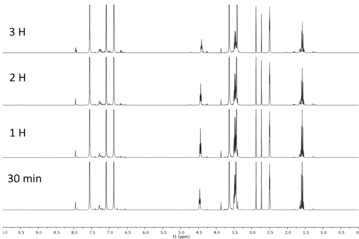
**Figure S21.** Kinetics of the depolymerisation of BPA-PC monitored through <sup>1</sup>H NMR spectroscopy carried out without catalyst, 1.05 eq. of 1,3-propanediol as nucleophile and 10 eq. of 1-Methylimidazole as solvent, after 3 h at 50 °C.
