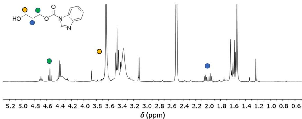
**Figure S24.**  $^1\text{H}$  NMR spectrum of the crude product of model reaction 2, 20 min after the addition of 1,3-propanediol. Reaction conditions: 1 eq. of imidazole as catalyst, 1.05 eq. of 1,3-propanediol as nucleophile and 10 eq. of 1-Methylimidazole as solvent, after 3 h at 50  $^\circ\text{C}$ .
