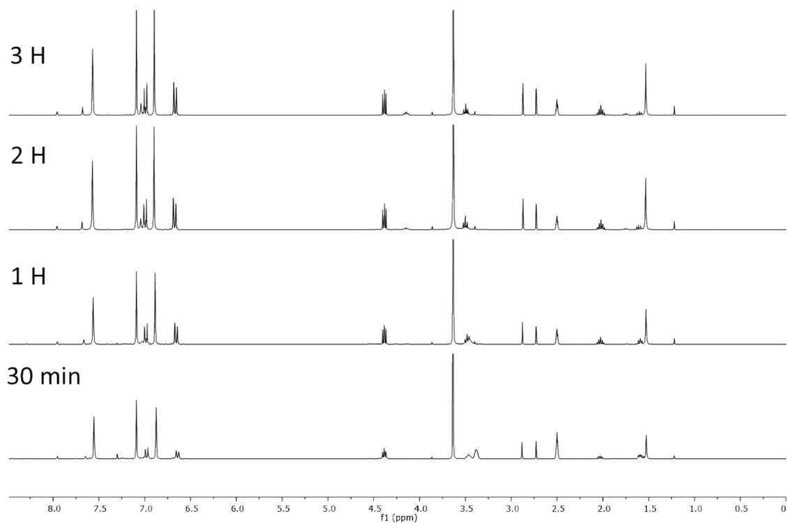
**Figure S15.** Kinetics of the depolymerisation of BPA-PC monitored through  $^1\text{H}$  NMR spectroscopy carried out with 1 eq. of imidazole as catalyst, 1.25 eq. of 1,3-propanediol as nucleophile and 10 eq. of 1-Methylimidazole as solvent, after 3 h at 50 °C.
