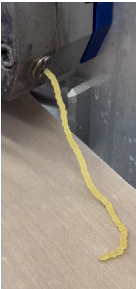
Figure S16. Extrusion of EOC CAN-38-1 at 200 °C. Note the surface defects from melt fracture.
