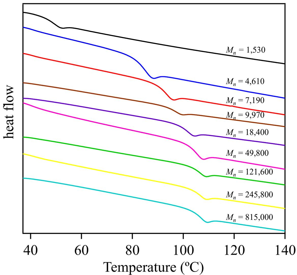
**Figure S16.** DSC curves of linear PS during the second heating (heating rate: 10 °C min<sup>-1</sup>).
