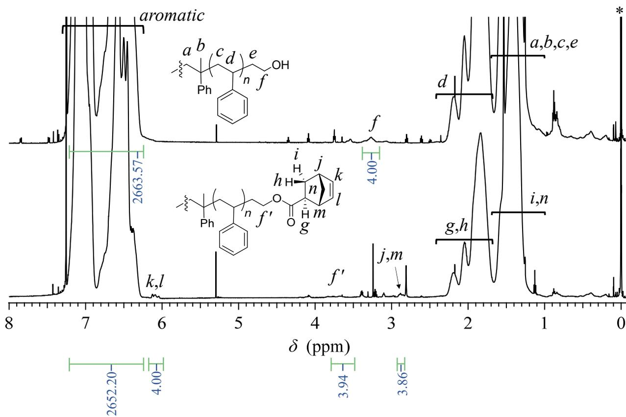
**Figure S6.** <sup>1</sup>H NMR spectra of HO-PS<sub>52k</sub>-OH (upper) and NB-PS<sub>52k</sub>-NB (lower) in CDCl<sub>3</sub>.
