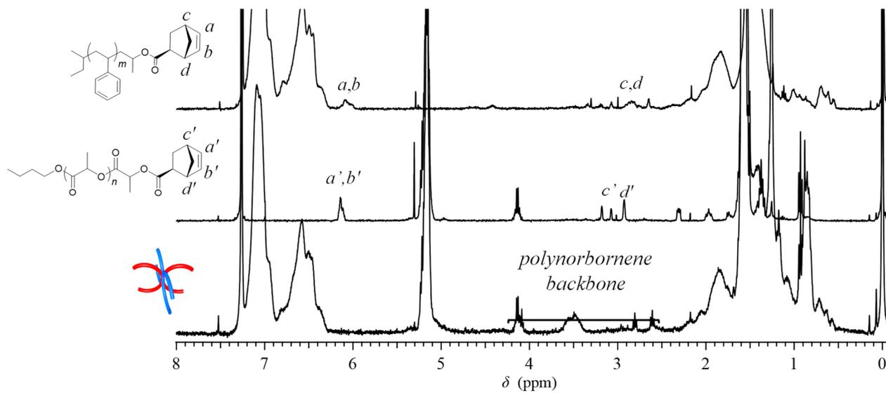
**Figure S25.**  $^1\text{H}$  NMR spectra of  $\text{PS}_{3\text{k}}\text{-NB}$  (upper),  $\text{PLA}_{3\text{k}}\text{-NB}$  (middle), and  $\text{poly}(\text{PS-}st\text{-PLA})$  (lower) in  $\text{CDCl}_3$ .
