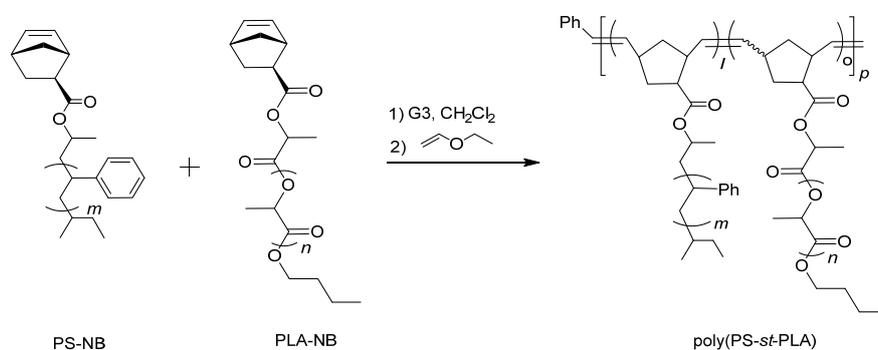
Method B was used for the ROMP of PS<sub>3k</sub>-NB (50.0 mg, 13.9  $\mu\text{mol}$ ) and PLA<sub>3k</sub>-NB (50.0 mg, 16.7  $\mu\text{mol}$ ) with G3 (316  $\mu\text{L}$ , 2.53  $\mu\text{mol}$  as a 8.0 mmol L<sup>-1</sup> solution in CH<sub>2</sub>Cl<sub>2</sub>) in dry CH<sub>2</sub>Cl<sub>2</sub> (1.52 mL) for 2.0 h to give poly(PS-*st*-PLA) as a brown solid. Yield: 76.7 mg (76.7%)
