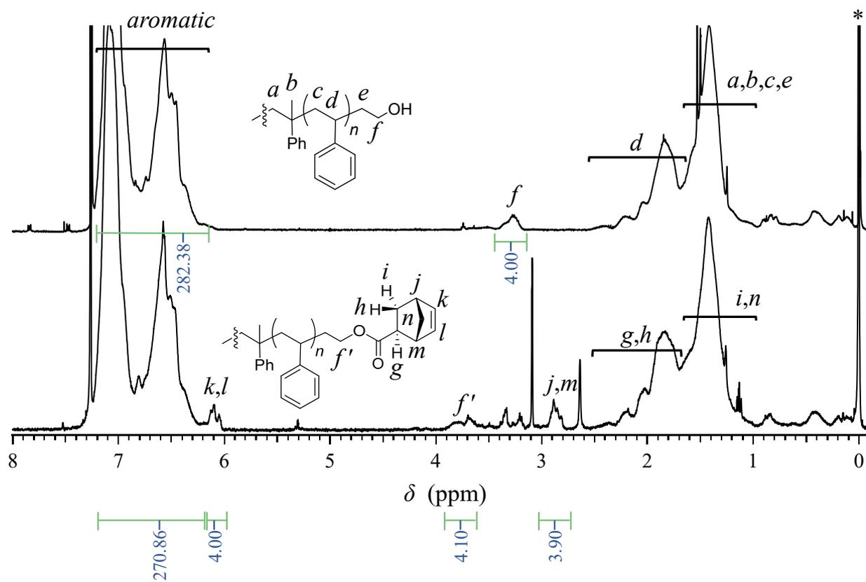
**Figure S3.**  $^1\text{H}$  NMR spectra of  $\text{HO-PS}_{6k}\text{-OH}$  (upper) and  $\text{NB-PS}_{6k}\text{-NB}$  (lower) in  $\text{CDCl}_3$ .
