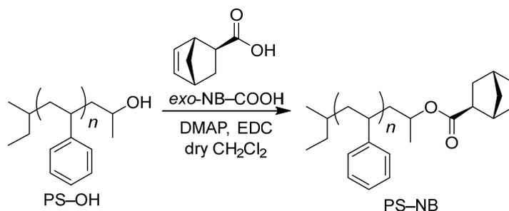
Method A was used for the reaction of PS-OH ( $M_{n,NMR} = 2,900$ , 2.30 g, 793  $\mu\text{mol}$ ) with *exo*-NB-COOH (268 mg, 1.94 mmol), DMAP (351 mg, 2.87 mmol), and EDC (559 mg, 2.92 mmol) in CH<sub>2</sub>Cl<sub>2</sub> (24 mL) for 4 days to give PS<sub>3k</sub>-NB as a white solid. Yield: 1.73 g (75.2%)
