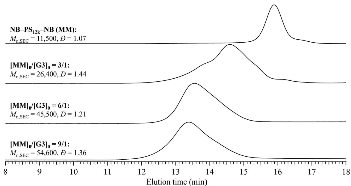
**Figure S9.** SEC traces of NB-PS<sub>12k</sub>-NB and *mc*-PS<sub>12k</sub> obtained from cyclopolymerization (refractive index (RI) detection; eluent, THF; flow rate, 1.0 mL min<sup>-1</sup>).
