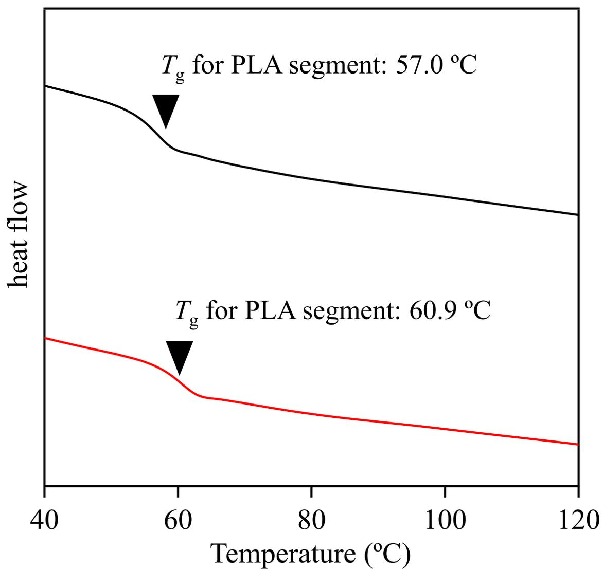
**Figure S19.** DSC curves during second heating process of NB-PLA-*b*-PS-*b*-PLA-NB (black) and *mc*-(PS-*b*-PLA) (run 15 in **Table S1**, red).
