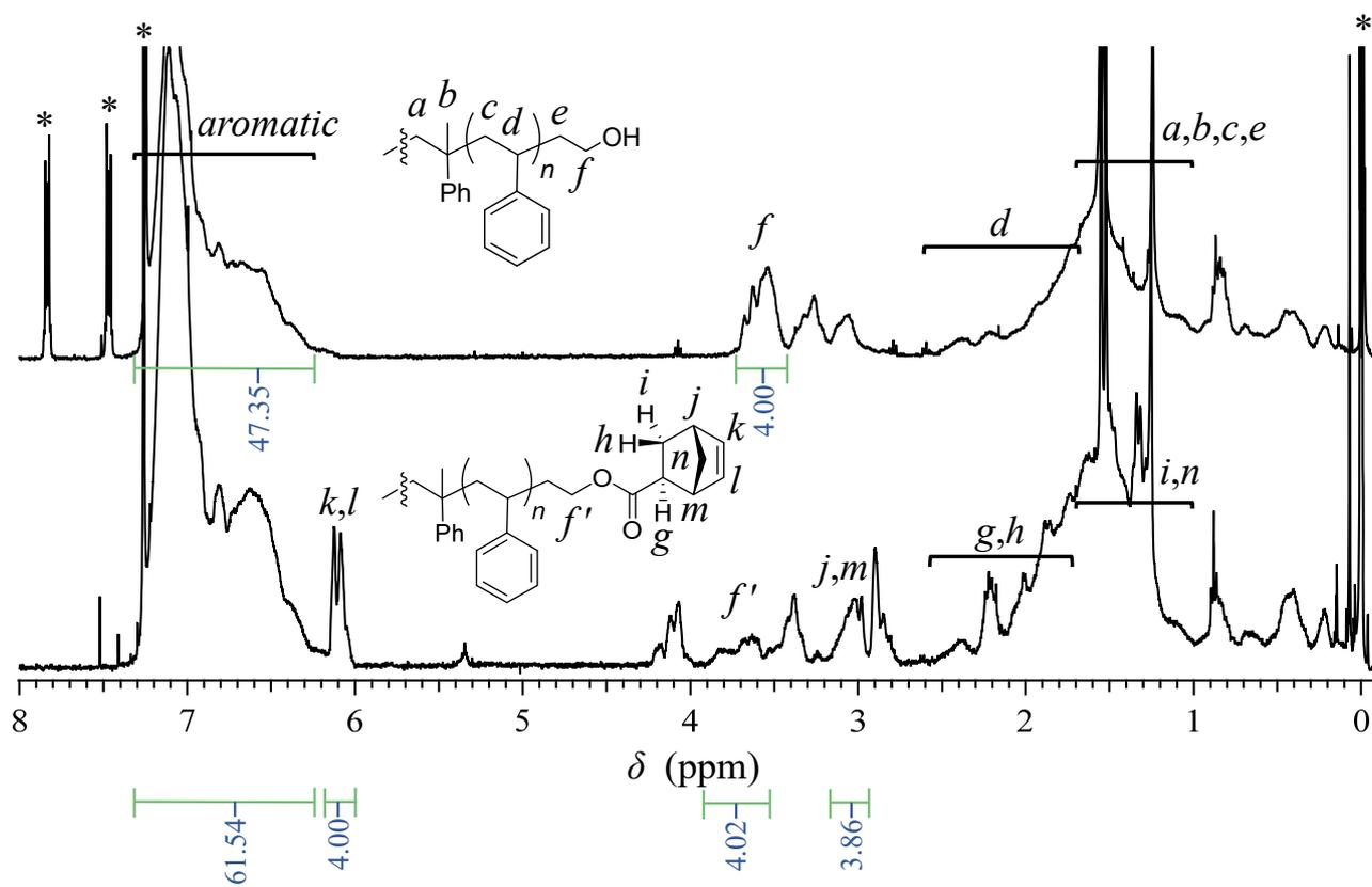
**Figure S2.** <sup>1</sup>H NMR spectra of HO-PS<sub>1k</sub>-OH (upper) and NB-PS<sub>1k</sub>-NB (lower) in CDCl<sub>3</sub>.
