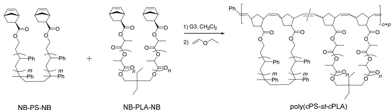
Method B was used for the ROMP of NB-PS<sub>6k</sub>-NB ( $M_{n,NMR} = 5,700$ , 50.0 mg, 8.77  $\mu\text{mol}$ ) and NB-PLA<sub>6k</sub>-NB ( $M_{n,NMR} = 6,700$ , 50.0 mg, 7.46  $\mu\text{mol}$ ) with G3 (1.01 mL, 8.06  $\mu\text{mol}$  as a 8.0  $\text{mmol L}^{-1}$  solution in  $\text{CH}_2\text{Cl}_2$ ) in dry  $\text{CH}_2\text{Cl}_2$  (129 mL) for 3h to give poly(*c*PS-*st*-*c*PLA) as a brown solid. Yield: 81.7 mg (81.7%)
