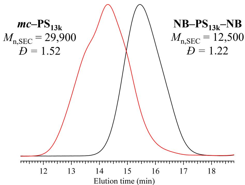
**Figure S13.** SEC traces of NB-PS<sub>13k</sub>-NB (black) and *mc*-PS<sub>13k</sub> (red) (RI detection; eluent, THF).
