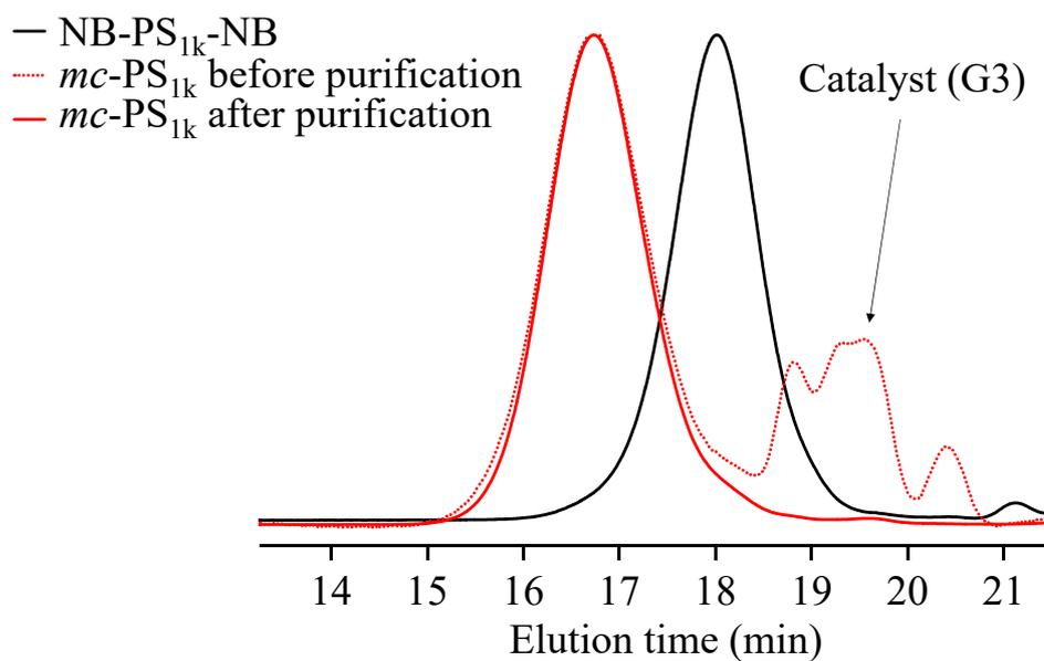
**Figure S1.** SEC traces of NB-PS<sub>1k</sub>-NB and *mc*-PS<sub>1k</sub> obtained from run 1 in **Table 2** before and after purification by preparative GPC (refractive index (RI) detection; eluent, THF; flow rate, 1.0 mL min<sup>-1</sup>).
