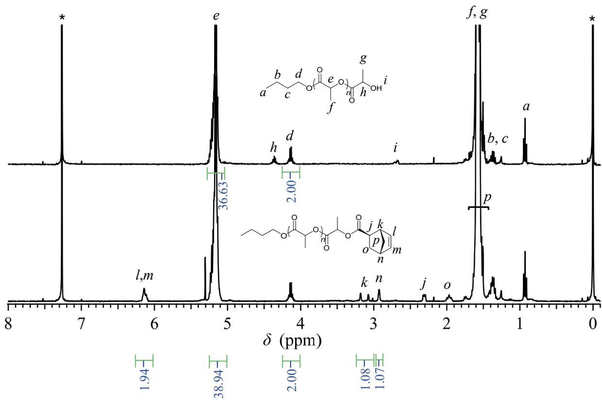
**Figure S24.** <sup>1</sup>H NMR spectra of PLA<sub>3k</sub>-OH (upper) and PLA<sub>3k</sub>-NB (lower) in CDCl<sub>3</sub>.
