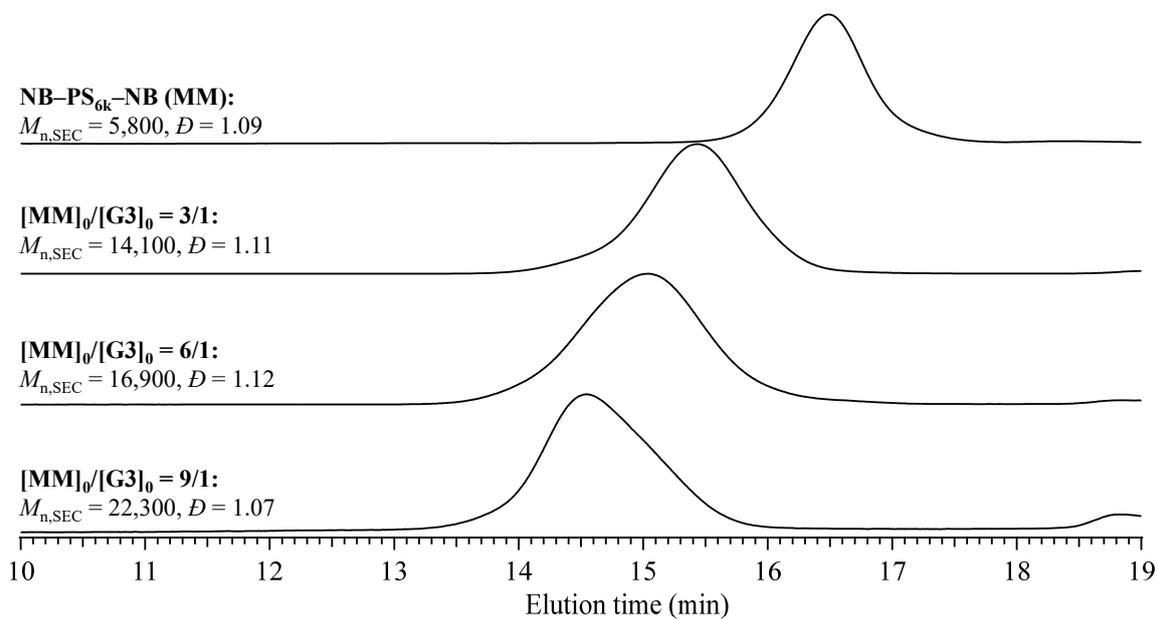
**Figure S8.** SEC traces of NB-PS<sub>6k</sub>-NB and *mc*-PS<sub>6k</sub> obtained from cyclopolymerization (refractive index (RI) detection; eluent, THF; flow rate, 1.0 mL min<sup>-1</sup>).
