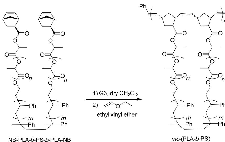
Method B was used for the ROMP of NB-PLA-*b*-PS-*b*-PLA-NB ( $M_{n,NMR} = 15,900$ , 50.0 mg, 3.14  $\mu\text{mol}$ ) with G3 (131  $\mu\text{L}$ , 1.04  $\mu\text{mol}$  as a 8.0 mmol L<sup>-1</sup> solution in CH<sub>2</sub>Cl<sub>2</sub>) in dry CH<sub>2</sub>Cl<sub>2</sub> (21.0 mL) for 1.5 h to give *mc*-(PLA-*b*-PS) as a brown solid. Yield: 49.8 mg (99.6%)
