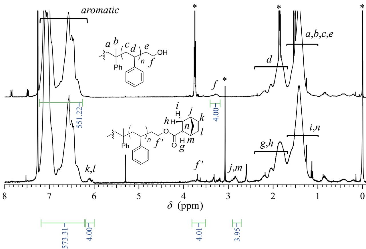
**Figure S5.** <sup>1</sup>H NMR spectra of HO-PS<sub>13k</sub>-OH (upper) and NB-PS<sub>13k</sub>-NB (lower) in CDCl<sub>3</sub>.
