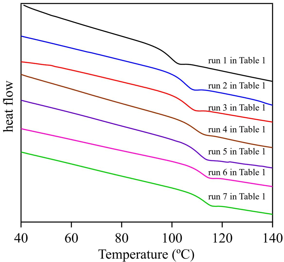
**Figure S15.** DSC curves of *mc*-PS<sub>1k</sub> during the second heating (heating rate: 10 °C min<sup>-1</sup>).
