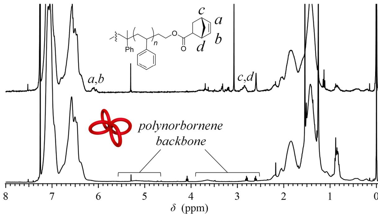
**Figure S14.** <sup>1</sup>H NMR spectra of NB-PS<sub>13k</sub>-NB (upper) and *mc*-PS<sub>13k</sub> (lower) in CDCl<sub>3</sub>.
