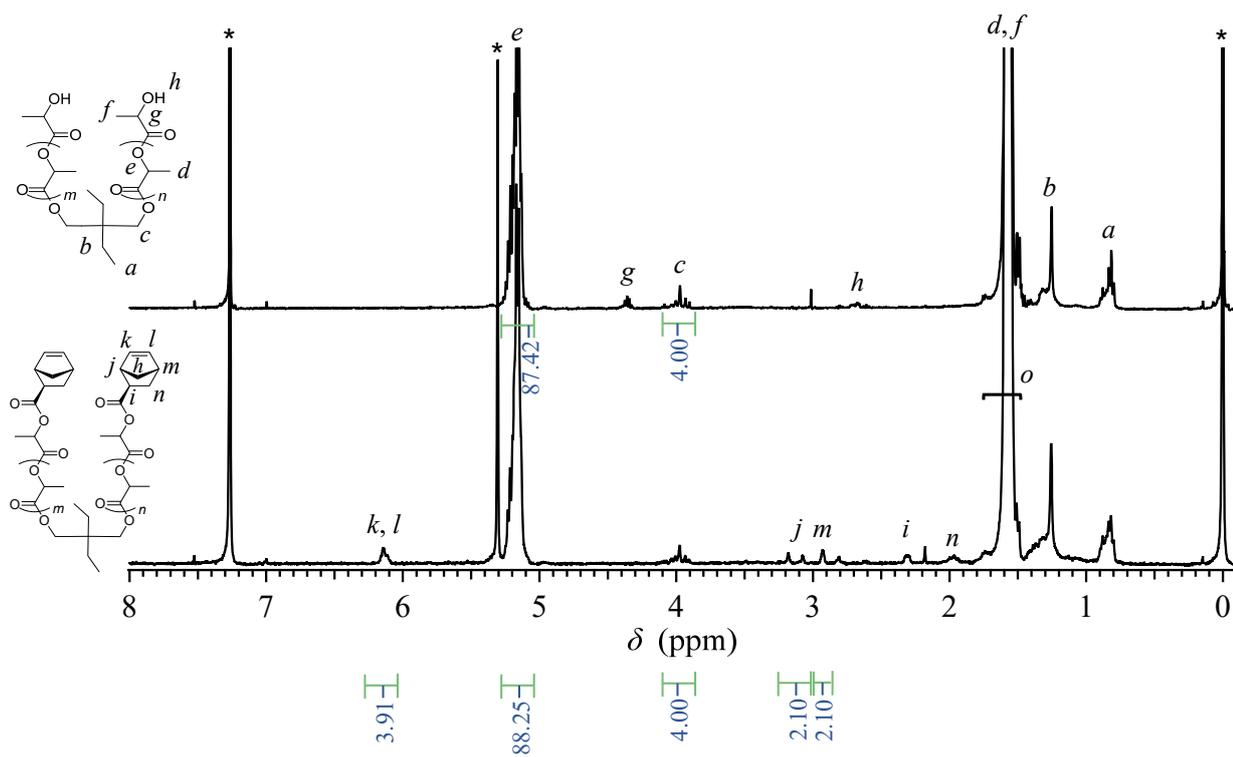
**Figure S20.**  $^1\text{H}$  NMR spectra of HO-PLA<sub>6k</sub>-OH (upper) and NB-PLA<sub>6k</sub>-NB (lower) in  $\text{CDCl}_3$ .
