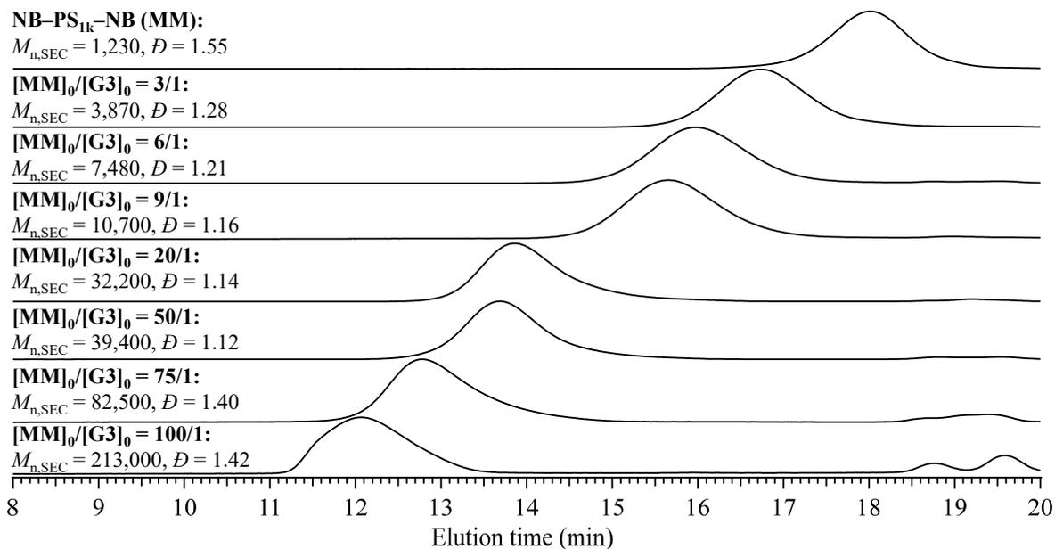
**Figure S7.** SEC traces of NB-PS<sub>1k</sub>-NB and *mc*-PS<sub>1k</sub> obtained from cyclopolymerization (refractive index (RI) detection; eluent, THF; flow rate, 1.0 mL min<sup>-1</sup>).
