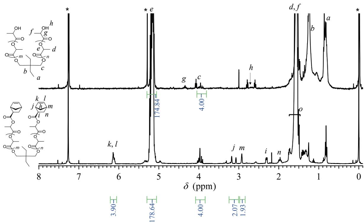
**Figure S21.** <sup>1</sup>H NMR spectra of HO-PLA<sub>13k</sub>-OH (upper) and NB-PLA<sub>13k</sub>-NB (lower) in CDCl<sub>3</sub>.
