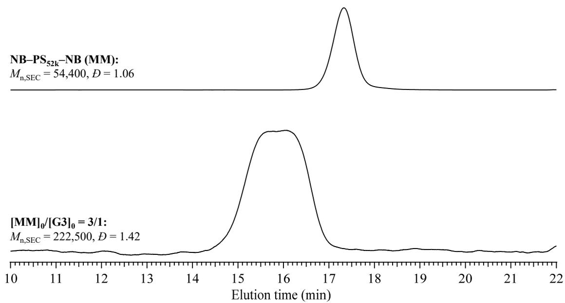
**Figure S12.** SEC traces of NB-PS<sub>52k</sub>-NB and *mc*-PS<sub>52k</sub> obtained from SEC with higher exclusion limit (refractive index (RI) detection; eluent, THF; flow rate, 1.0 mL min<sup>-1</sup>).
