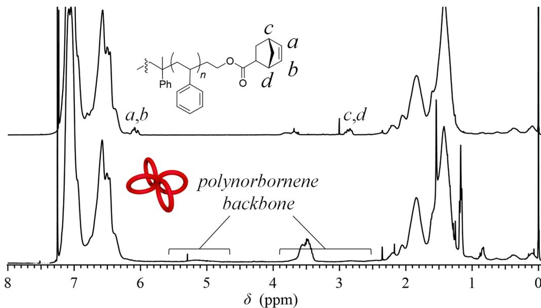
**Figure S11.**  $^1\text{H}$  NMR spectra of NB-PS<sub>12k</sub>-NB (upper) and mc-PS<sub>12k</sub> (run 11 in Table 2, lower) in CDCl<sub>3</sub>.
