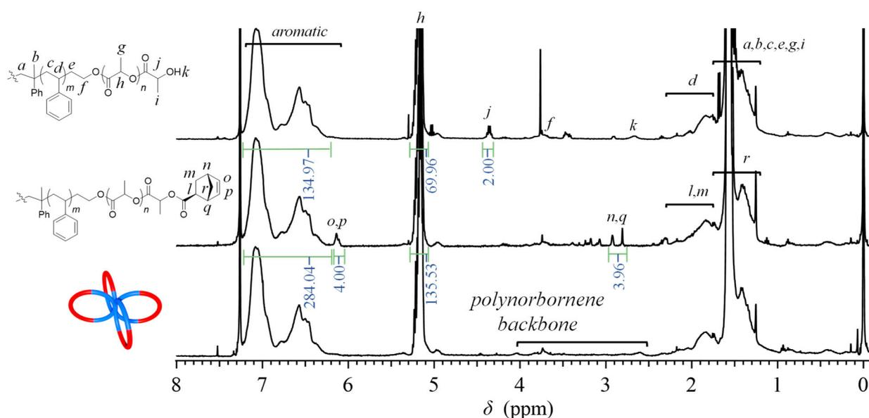
**Figure S18.** <sup>1</sup>H NMR spectra of HO-PLA-*b*-PS-*b*-PLA-OH (upper), NB-PLA-*b*-PS-*b*-PLA-NB (middle), and *mc*-(PLA-*b*-PS) (lower) in CDCl<sub>3</sub>.
