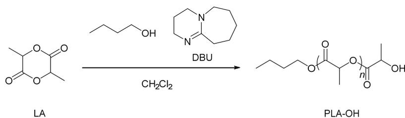
Method A was used for the polymerization of LA (1.50 g, 10.4 mmol) with 1-butanol (29.6 mg, 399  $\mu$ mol) and DBU (15.9  $\mu$ L, 104  $\mu$ mol) in CH<sub>2</sub>Cl<sub>2</sub> (10.4 mL) for 1 min to give PLA<sub>3k</sub>-OH as a white solid. Yield: 859 mg (69.3%)
