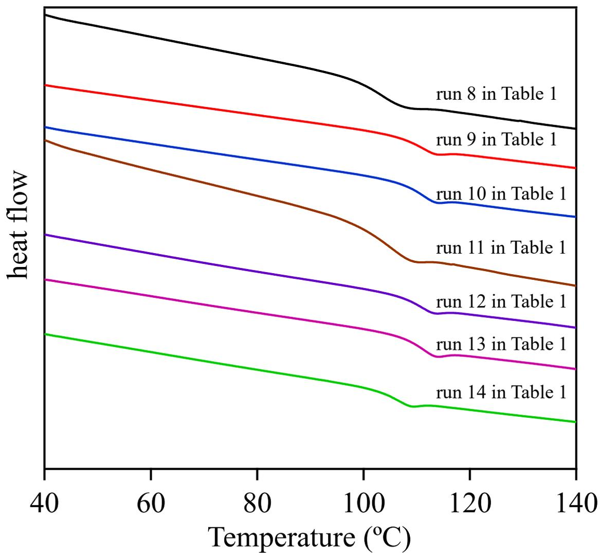
**Figure S17.** DSC curves of *mc*-PS<sub>6k</sub>, *mc*-PS<sub>12k</sub>, and *mc*-PS<sub>52k</sub> during the second heating (heating rate: 10 °C min<sup>-1</sup>).
