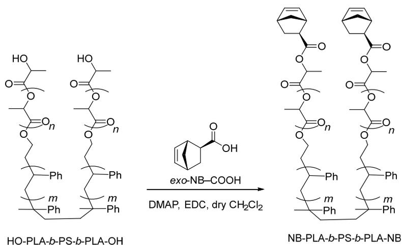
Method A was used for the reaction of HO-PLA-*b*-PS-*b*-PLA-OH ( $M_{n,NMR} = 16,000$ , 1.00 g, 62.5  $\mu\text{mol}$ ) with *exo*-NB-COOH (34.5 mg, 249  $\mu\text{mol}$ ), DMAP (45.8 mg, 375  $\mu\text{mol}$ ), and EDC (485 mg, 375  $\mu\text{mol}$ ) in CH<sub>2</sub>Cl<sub>2</sub> (10.0 mL) for 81 h to give NB-PLA-*b*-PS-*b*-PLA-NB as a white solid. Yield: 831 mg (83.1%)
