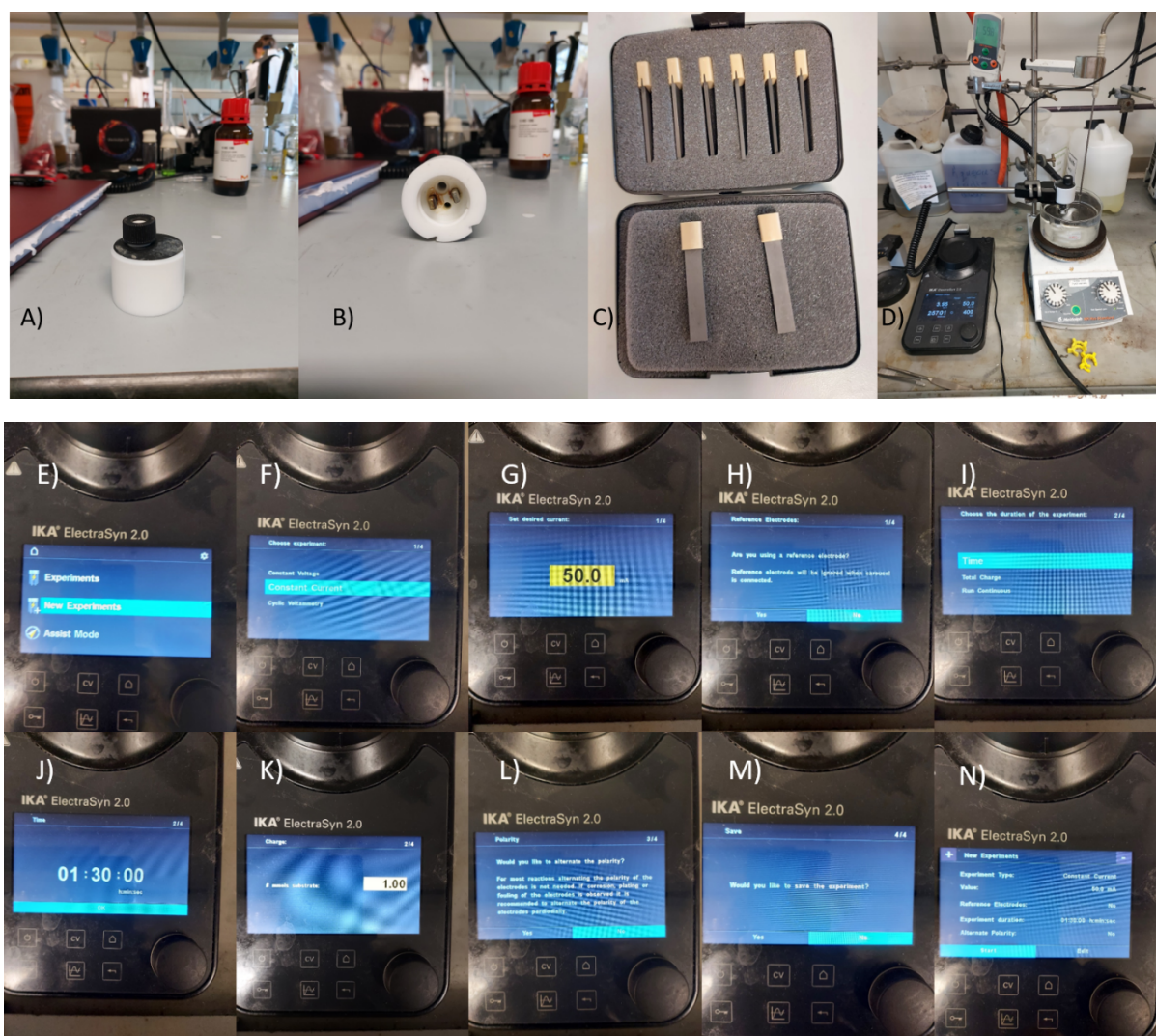
Fig. S1 IKA ElectraSyn 2.0 device configuration for the eHoffman reaction. A and B) IKA head/cap; C) IKA graphite electrodes; D) fully assembled reaction using the IKA ElectraSyn GoGo module to enable the reaction to be heated in an oil bath. Direction for setting up the reaction using the ElectraSyn interface includes E) select new experiment; F) choose constant current electrolysis (CCE); G) use the dial to set I_{app} (50 mA in our hands); H) press 'no' if no reference electrode is required (which is the case for CCE); I) select the 'Time'; J) use the dial to set the reaction time (1 h 30 min 00 sec in this case); K) use the dial to set the substrate concentration (1 mmol in this case); L) select 'no' to alternating polarity; M) choose whether to save the data or not; N) press start.
