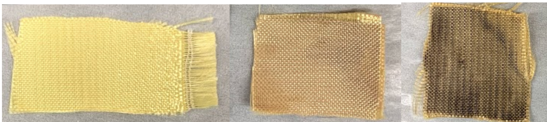
Figure 5. Comparison of plain Kevlar (left), Kevlar with dye treatment (center), Kevlar with diazirine treatment then dye treatment (right).
