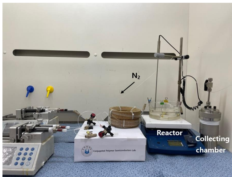
Figure S1. An image of the flow synthesis system used in this study.
