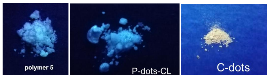
Figure S3. Fluorescent behaviors of PMAA- b -PMMA and crosslinked polymer dots with different polymer weight in solid state under a UV light ( \lambda_{\text{ex}}=365 nm).
