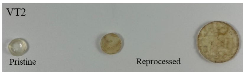
Fig. S48: Picture representing pristine VT2 (left) and the reprocessed counterparts (right)
