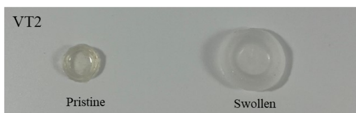
Fig. S36: Picture representing pristine VT2 (left) and the swollen in CH_2Cl_2 counterpart (right)
