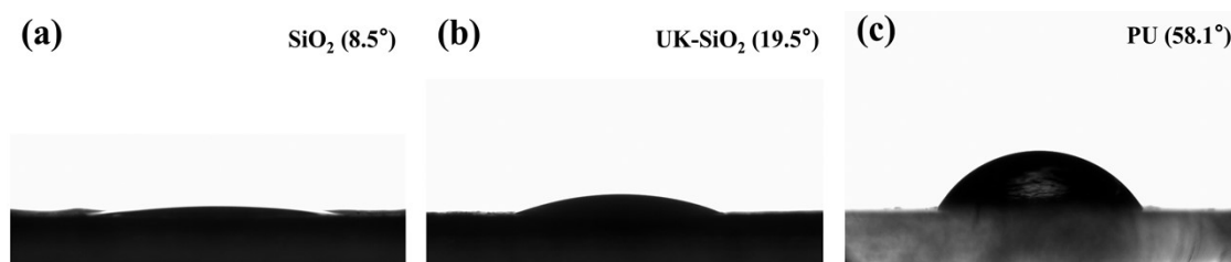
Fig. S5. (a) Photo of water contact angle of nano-SiO 2 ; (b) photo of water contact angle of UK-SiO 2 ; (c) photo of water contact angle of PU.
