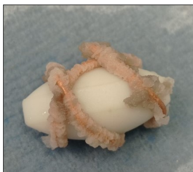
Figure S12: Image of the copper catalyst at the end of the SET-LR-PISA reaction when targeting DP_{HPMA} = 450 . Gelation of the polymer around the copper wire catalyst was observed.
