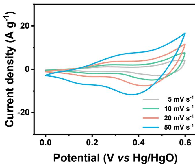
**Figure S10.** CV curves of H-Co<sub>9</sub>S<sub>8</sub> measured in 1M KOH at the range of current densities between 5 – 50 mV s<sup>-1</sup>.
