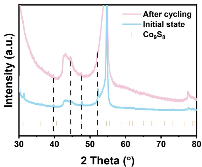
**Figure S9.** XRD patterns of S-Co<sub>9</sub>S<sub>8</sub> before and after the alkaline OER test.
