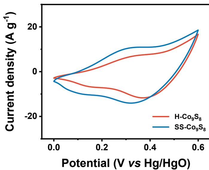
**Figure S11.** The comparison of CV curves was measured at  $50 \text{ mV s}^{-1}$  for S- $\text{Co}_9\text{S}_8$  and H- $\text{Co}_9\text{S}_8$ .
