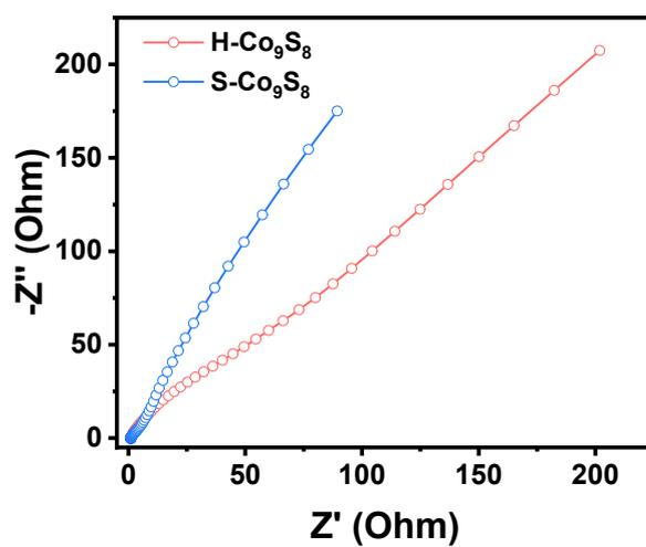
**Figure S14.** Nyquist plots for S-Co<sub>9</sub>S<sub>8</sub> and H-Co<sub>9</sub>S<sub>8</sub>.
