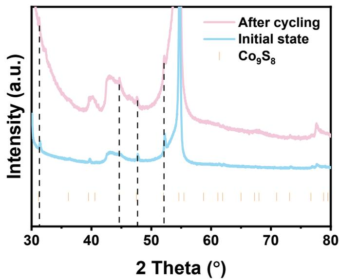
**Figure S6.** XRD patterns of S-Co<sub>9</sub>S<sub>8</sub> before and after the cycling stability test in acidic HER.
