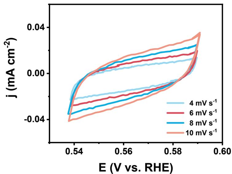
**Figure S3.** CV curves of S-Co<sub>9</sub>S<sub>8</sub> at different sweep rates in 0.5 M H<sub>2</sub>SO<sub>4</sub>.
