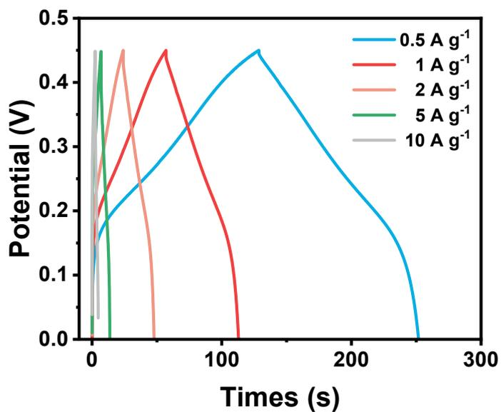
**Figure S12.** GCD curves under various current densities of the H- $\text{Co}_9\text{S}_8$  electrode by using  $1 \text{ mol L}^{-1}$  KOH aqueous electrolyte.
