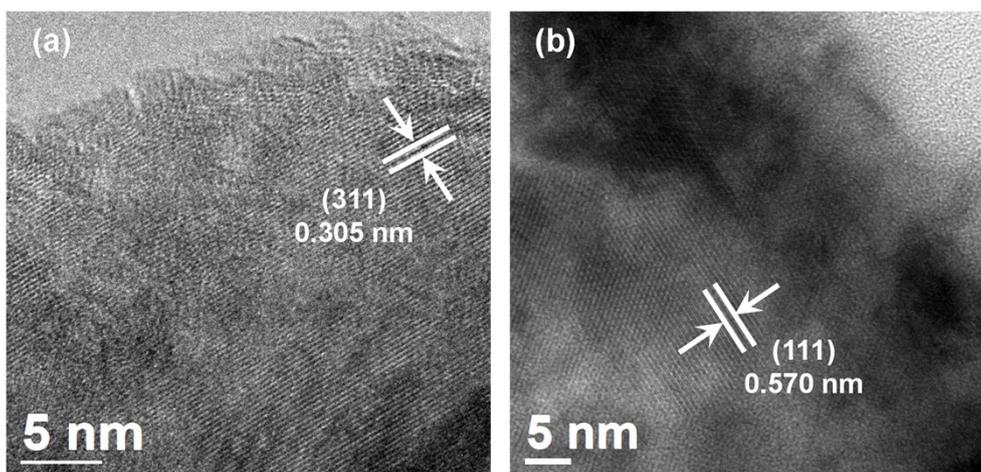
**Figure S2.** HRTEM images of (a) S-Co<sub>9</sub>S<sub>8</sub> and (b) H-Co<sub>9</sub>S<sub>8</sub>.
