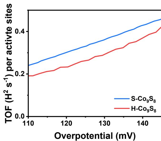
**Figure S5.** TOF values of S-Co<sub>9</sub>S<sub>8</sub> and H-Co<sub>9</sub>S<sub>8</sub> electrodes.
