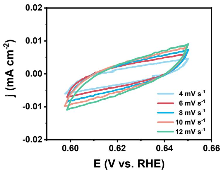
**Figure S4.** CV curves of H-Co<sub>9</sub>S<sub>8</sub> at different sweep rates in 0.5 M H<sub>2</sub>SO<sub>4</sub>.
