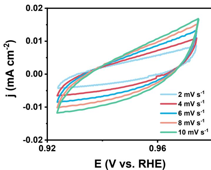
**Figure S7.** CV curves of S-Co<sub>9</sub>S<sub>8</sub> at different sweep rates in 1 M KOH.
