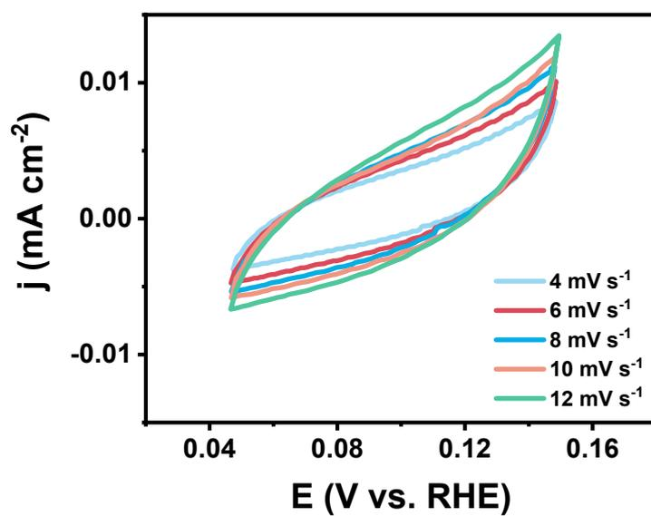
**Figure S8.** CV curves of H-Co<sub>9</sub>S<sub>8</sub> at different sweep rates in 1 M KOH.
