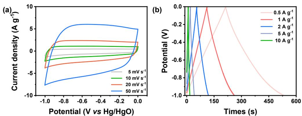
**Figure S13.** CV curves and GCD curves of the YP-50 electrode by using 1 mol L<sup>-1</sup> KOH aqueous electrolyte.
