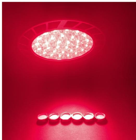
**Figure S14.** Real scenes of optical excitation of ZLGGC samples under the irradiation by  $\sim 740$  nm NIR LED.
