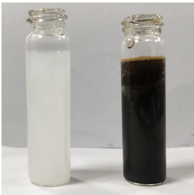
Figure S61. Change in colour of Hf-UiO-66-NHCSNHCH 3 + \text{Pb}(\text{CH}_3\text{COO})_2 aqueous mixture after the addition of \text{NH}_2\text{-NH}_2 .
