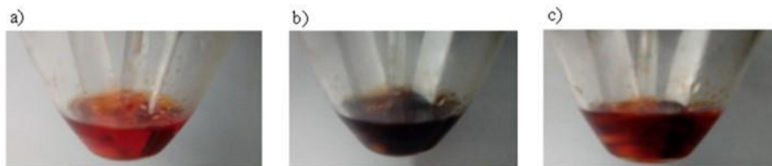
Figure S9. Colour change observation from orange (a) (before electrolysis) to brown (b) (after electrolysis). After air injection into the solution colour reverts back to orange (c).
