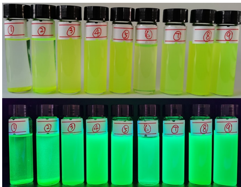
Figure S3. Photograph show the PFGA-CsPbBr 3 NCs in different solvents, including n-hexane, toluene, ethyl acetate, acetone, tert-butanol, isopropanol, ethanol, acetonitrile, from left to right under normal white light (up) and a 365 nm UV (down).
