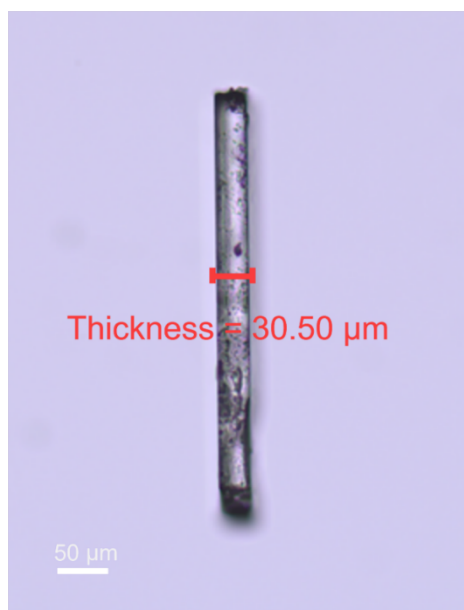
Figure S6 The thickness of the selected RPNCO single-crystal used for the birefringence measurement.
