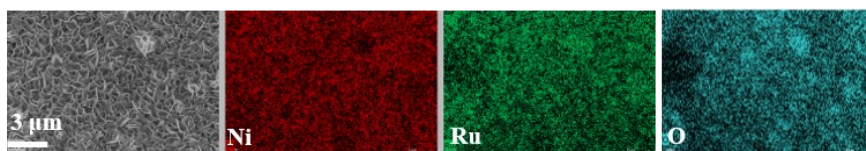
Figure S2. SEM images and elemental mapping of \text{Ni}_2\text{Ru}(\text{OH})_x .
