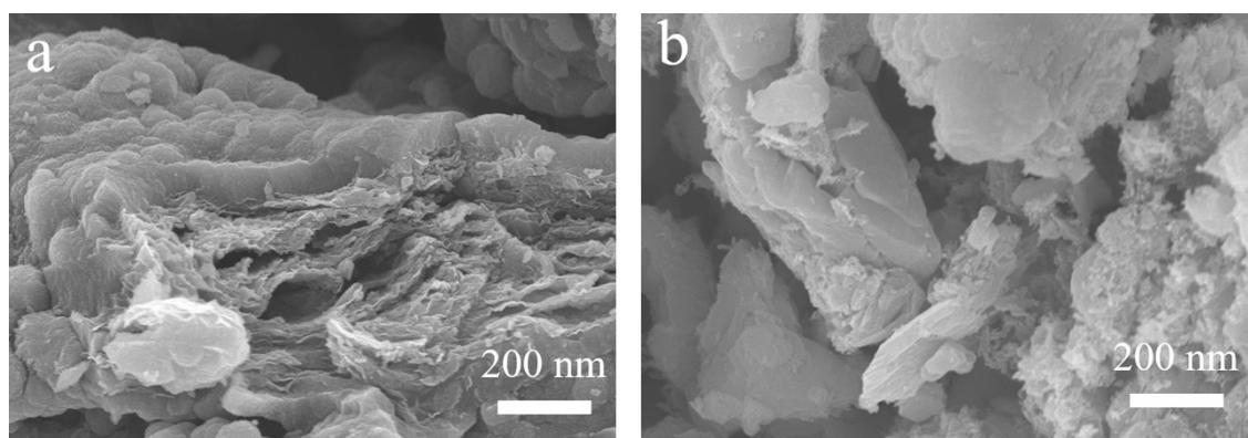
**Fig. S12** SEM images of AlHCF/Gr a) before and b) after 200 cycles.
