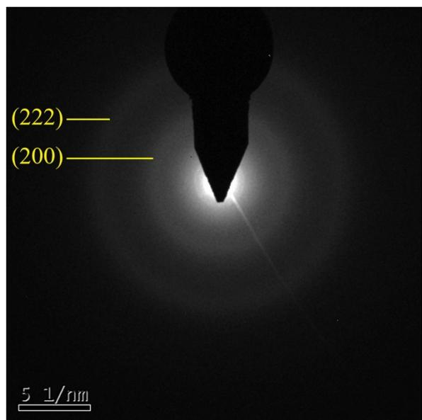
**Fig. S5** The selected area electron diffraction (SAED) patterns of AlHCF. The diffraction ring of AlHCF confirms its polycrystalline characteristics.
