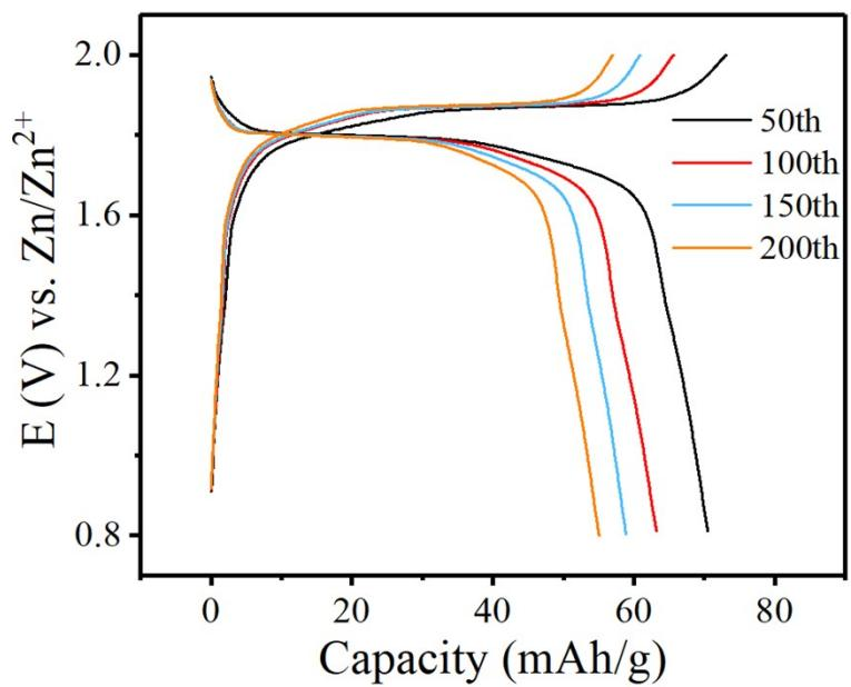
**Fig. S8** GCD profiles of long-term cycle.
