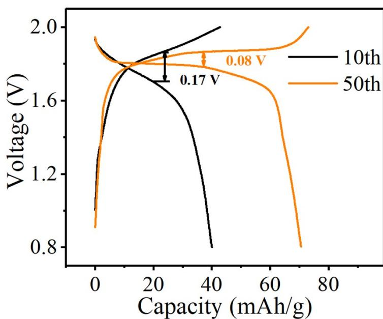
**Fig. S7** Voltage difference between the charge and discharge plateaus of cycle 10 and cycle 50.
