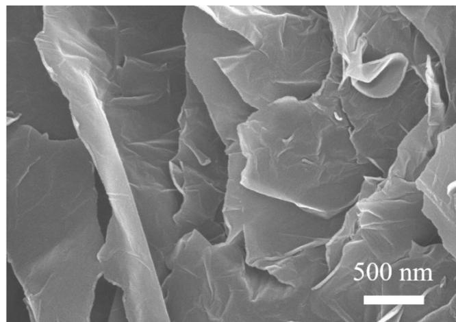
**Fig. S1** Graphene sheet obtained through thermal exfoliation of graphene oxide.
