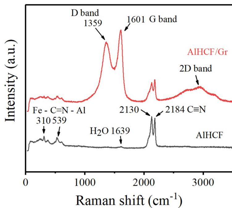
**Fig. S3** Raman spectra of AlHCF and AlHCF/Gr.
