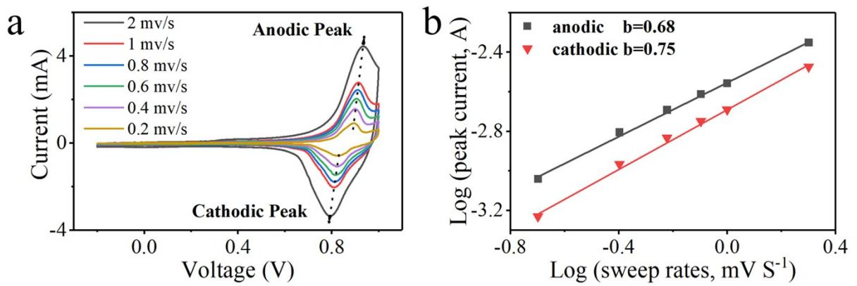
**Fig. S11** Electrode kinetics analysis of AlHCF/Gr electrode with cycling. a) Cyclic voltammograms of AlHCF at various scan rates. b)  $\log(i)$  -  $\log(v)$  plots of anodic and cathodic peaks derived from the scan rate dependent CV curves.
