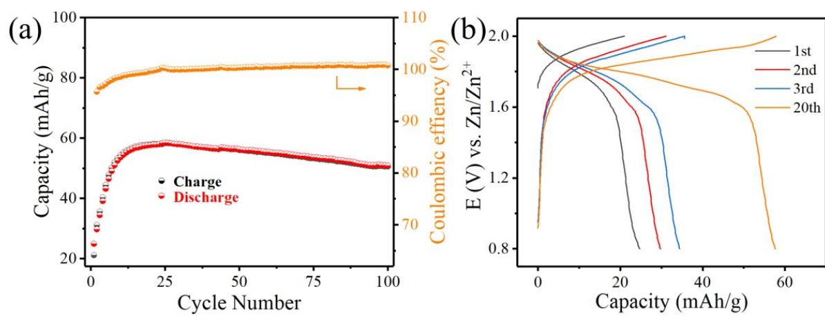
**Fig. S10** Electrochemical performance of full cell at 5C (1C=60 mA g<sup>-1</sup>). a) Cycling performance of full cell using AlHCF/Gr as cathode. b) GCD profiles of full cell.
