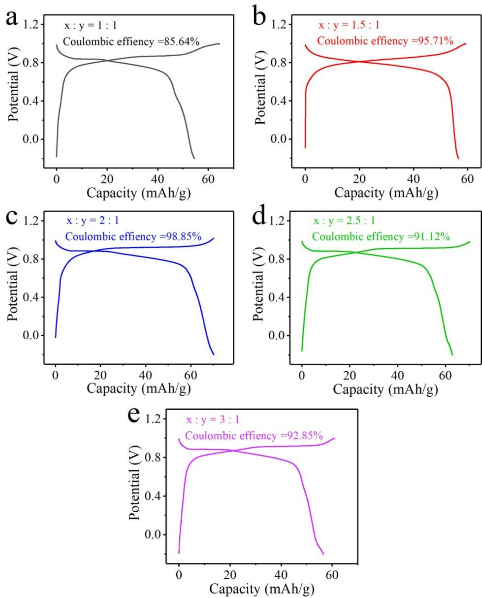
**Fig. S6 a-e)** Galvanostatic charge/discharge (GCD) profiles at maximum capacity for different ingredient proportion of AlHCF, x:y represents the ingredient proportion of  $\text{Al}^{3+} : \text{Fe}(\text{CN})_6^{4-}$ .
