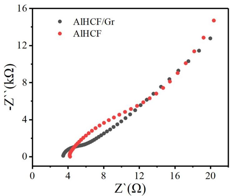
**Fig. S9** Electrochemical impedance spectroscopy (EIS) of AlHCF and AlHCF/Gr.
