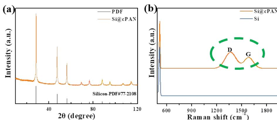
**Figure S1.** (a) XRD patterns of Si@cPAN. (b) Raman spectra of Si and Si@cPAN.
