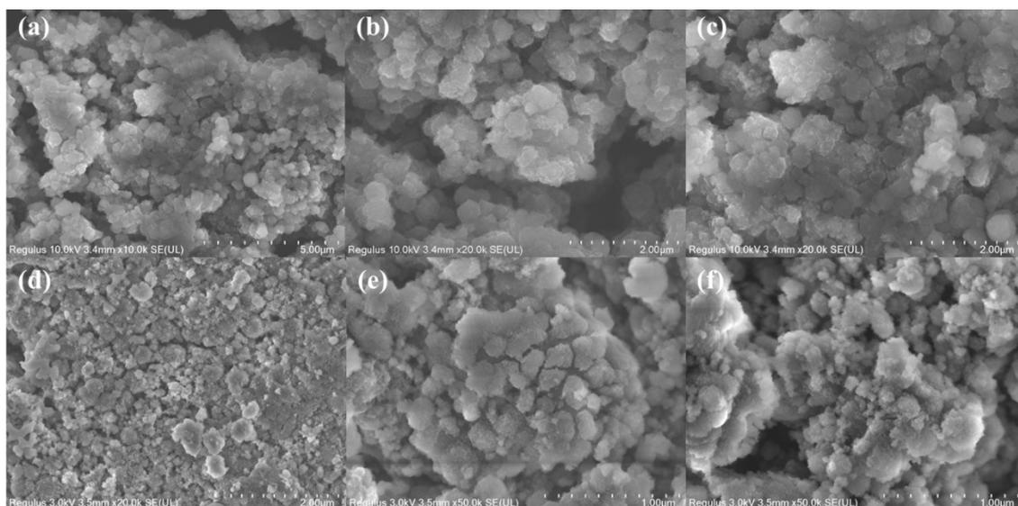
**Figure S7.** SEM images of (a-c) Si@cPAN@CMC and (d-f) Si@CMC particles after 50 cycles at  $1 \text{ A g}^{-1}$
