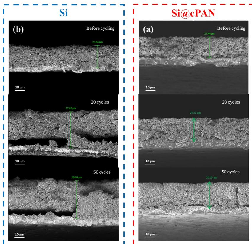
**Figure S6.** Cross-sectional SEM images of (a) Si@cPAN@CMC electrodes (b) Si@CMC electrodes before cycling and after 20 and 50 cycles at  $1 \text{ A g}^{-1}$
