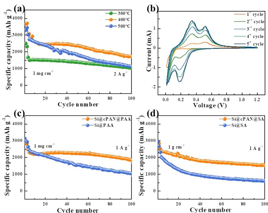
**Figure S2.** (a) Cycling performance of Si@cPAN@CMC electrodes treated at 300°C, 400°C, 500°C at  $2 \text{ A g}^{-1}$  for 100 cycles. (b) CV curves of Si@cPAN@CMC electrode for different cycles. Cycling performance of (c) Si@PAA and Si@cPAN@PAA
