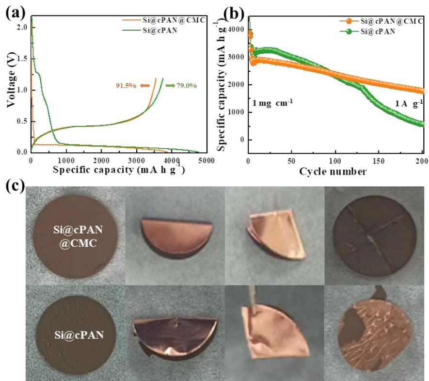
**Figure S4.** (a) The charge-discharge profiles and (b) cycling performances of Si@cPAN@CMC and Si@cPAN electrodes for 200 cycles. (c) Electrode photo of Si@cPAN@CMC and Si@cPAN electrodes with a mass loading of  $3.0 \text{ mg cm}^{-2}$
