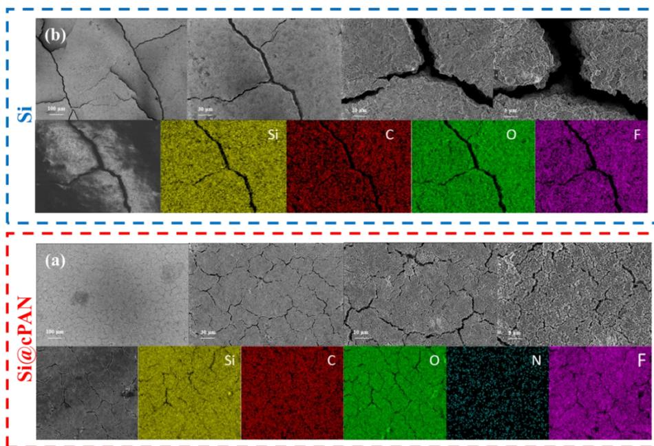
**Figure S5.** SEM images and corresponding EDS mappings of (a) Si@CMC and (b) Si@cPAN@CMC electrodes after 50 cycles at  $1 \text{ A g}^{-1}$
