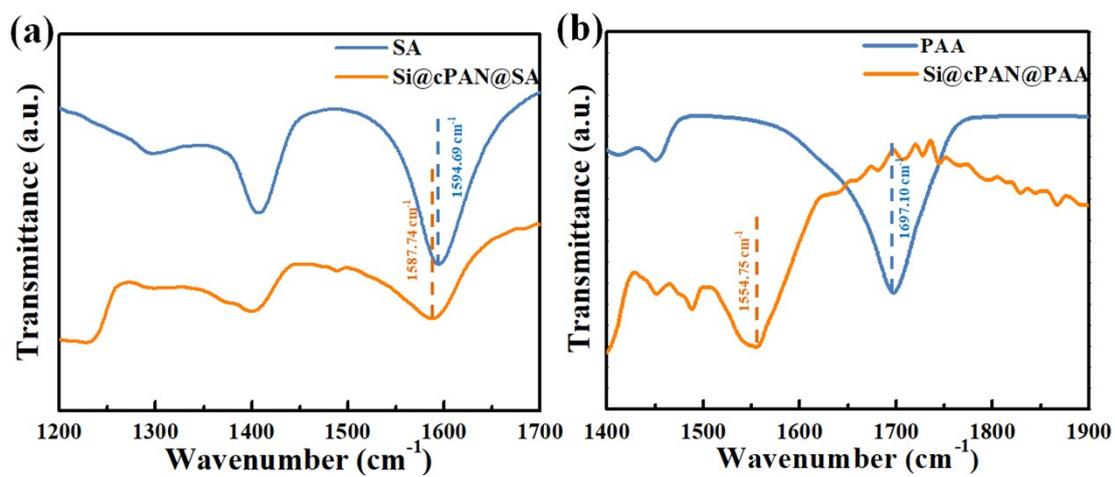
**Figure S9.** FTIR spectra of (a) SA and Si@cPAN@SA, (b) PAA and Si@cPAN@PAA electrode.
