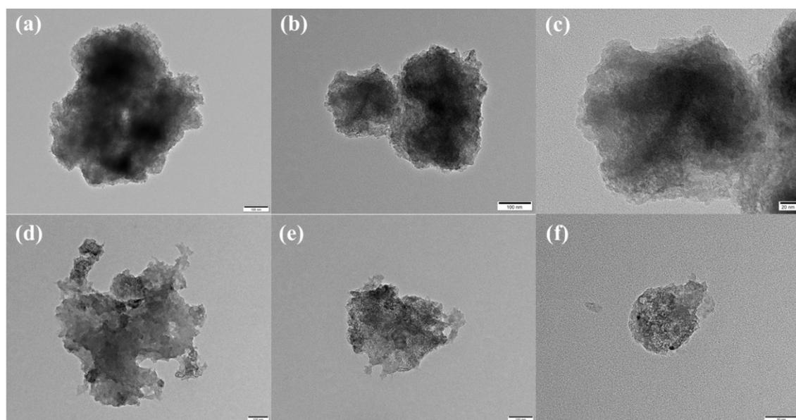
**Figure S8.** TEM images of (a-c) Si@cPAN@CMC and (d-f) Si@CMC particles after 50 cycles at  $1 \text{ A g}^{-1}$
