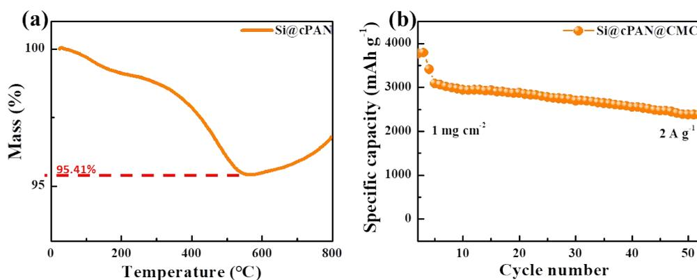
**Figure S3.** (a) TG curve of Si@cPAN particles. (b) Cycling performance of the Si@cPAN@CMC electrode by mixing Si@cPAN, carbon black, and CMC with a mass ratio of 8.4:1:0.6 .
