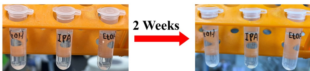
Figure S18. Comparison of the solubility of \text{CuBr} in methanol, ethanol, and isopropanol.
