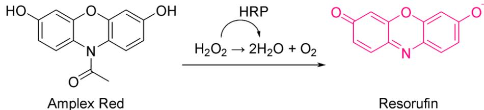
**Figure S1.** Reaction between Amplex Red and  $\text{H}_2\text{O}_2$  in a 1:1 stoichiometry in the presence of horseradish peroxidase (HRP), generating resorufin with a UV-vis absorption band at 571 nm.
