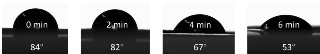
Fig. S6 Water contact angle of the RGO/CNFs@PPy-20 at different times.
